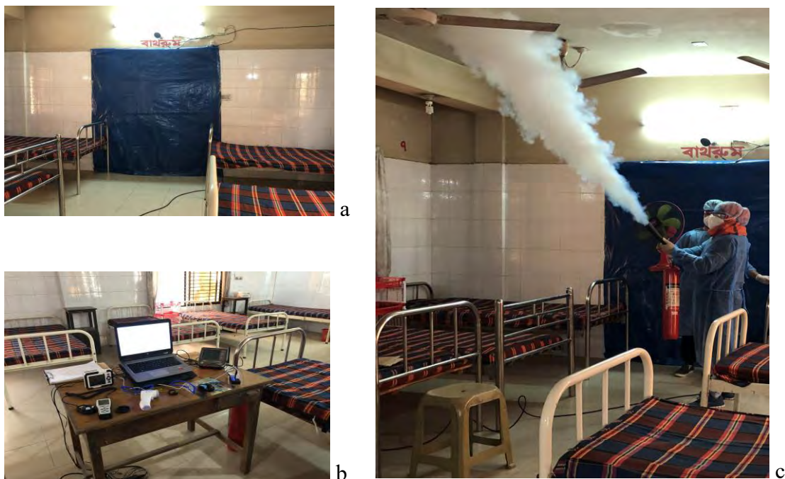
Figure 5-3: (a) Corridor covered with polythene sheets, (b) instrument set up, (c) injecting CO 2
