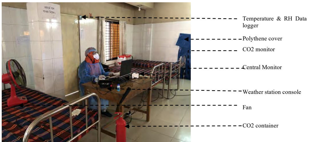
Figure 5-2: The interior view of the measured hospital ward showing fans, instruments, and CO 2 bottles
