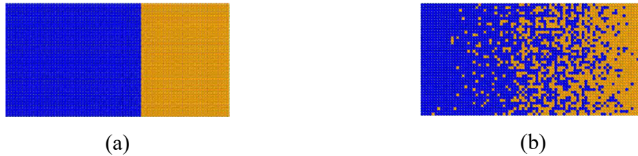
Figure 4.3: Atomistic configuration of the (a) patterned (b) FWG hybrid wetting surface with fraction of hydrophilic atoms, \alpha = 0.6 .
