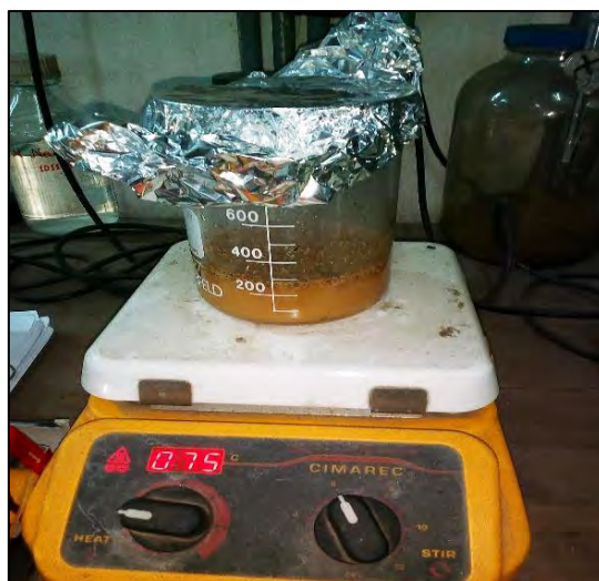
Figure 3.7: Wet Peroxide Oxidation using hotplate
