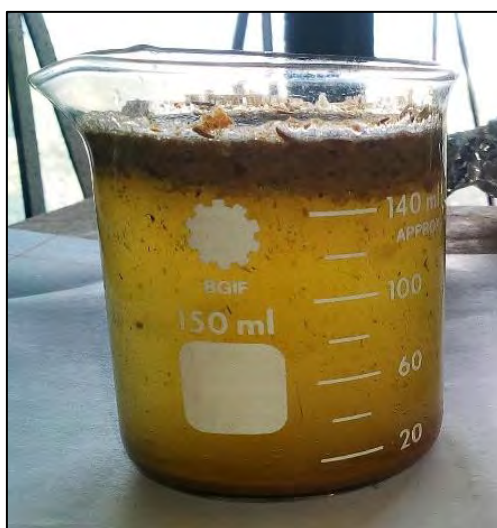
Figure 3.8: Density separation of sample to separate microplastics
