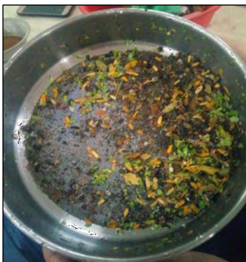
Figure 3.5: A sample retained on No. 50 sieve (after sieving and rinsing)
