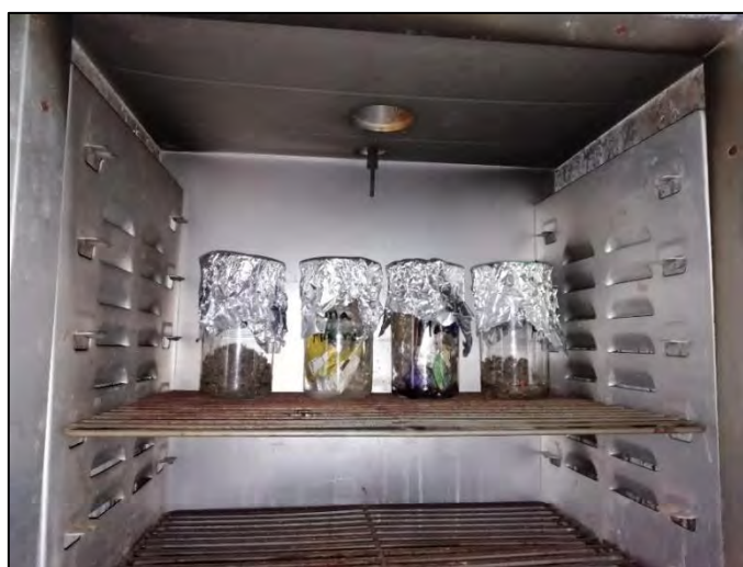
Figure 3.6: Oven dry samples to determine dry weight
