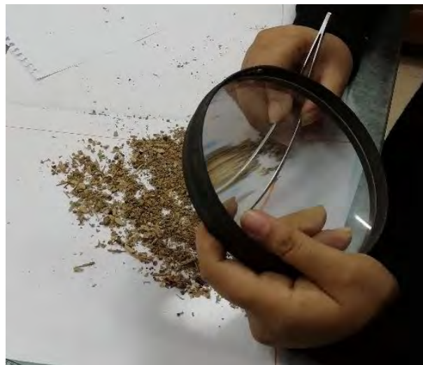
Figure 3.10: Microplastics fragments separation using magnifying glass
