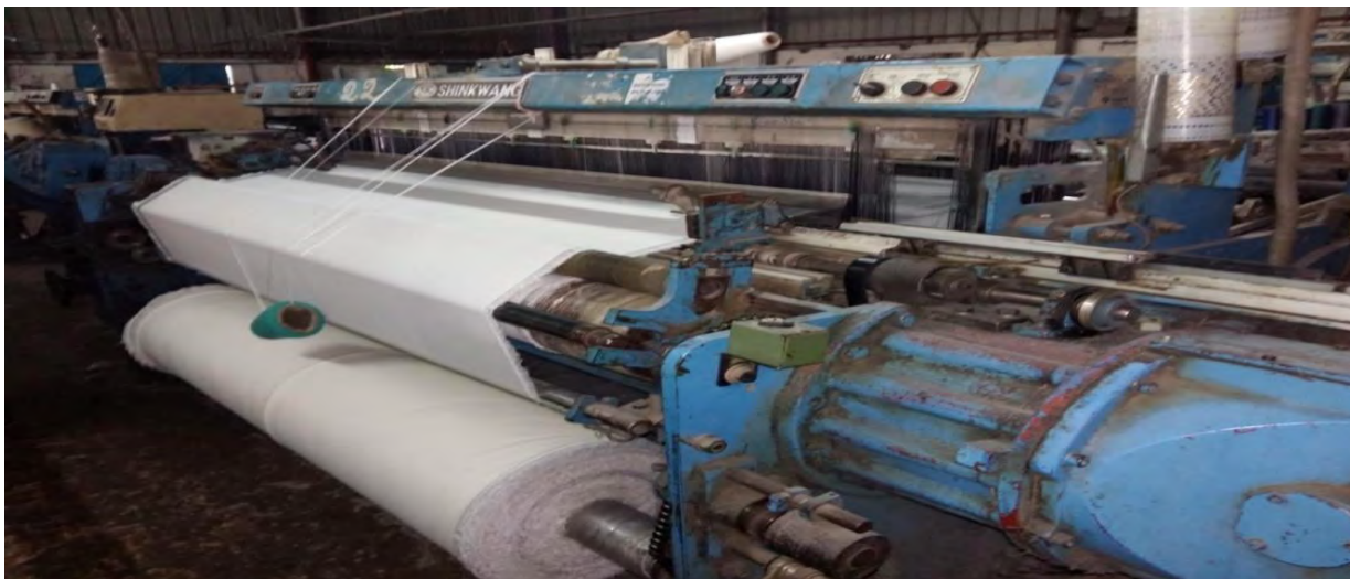
Figure 2.2: Shinkwang machine for producing cloth from yarn.
