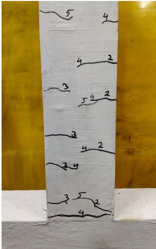
Figure 4.5: (a) Cracks in specimen 5-BSS-B (b) Failure zone of specimen 5-BSS-B
