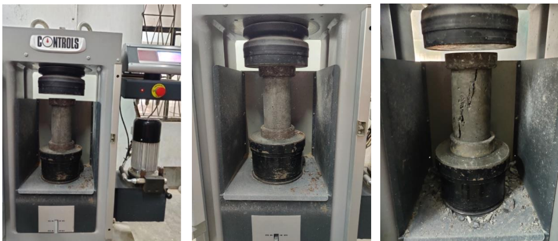
Figure 3.12: Compressive strength test of concrete cylinders
