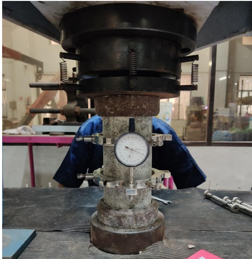
Figure 3.13: Stress versus strain test of concrete
