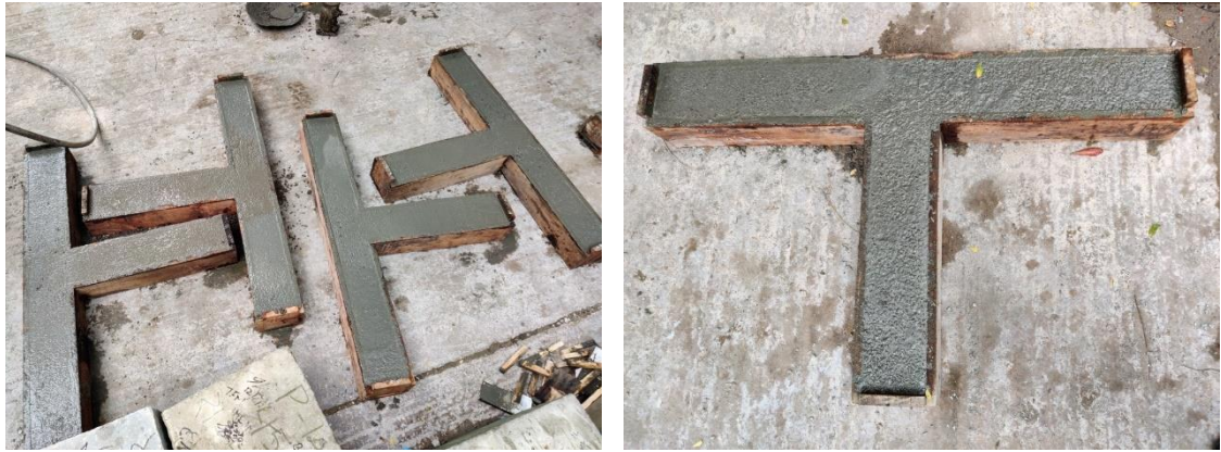
Figure 3.23: Specimens after fresh concrete is cast
