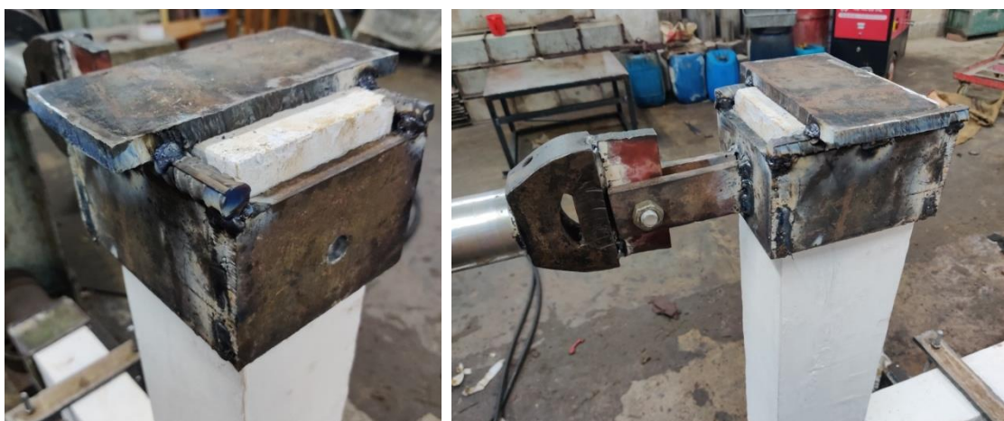
Figure 3.28: Customized steel collar at beam end
