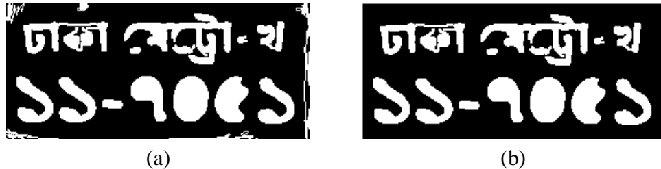
Figure 4.35: Illustration of the MATLAB function imclearborder to remove border pixels of (a) an image to (b) a cleared one
