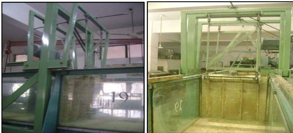
Figure 3.3(b): Photo views of wave generator
