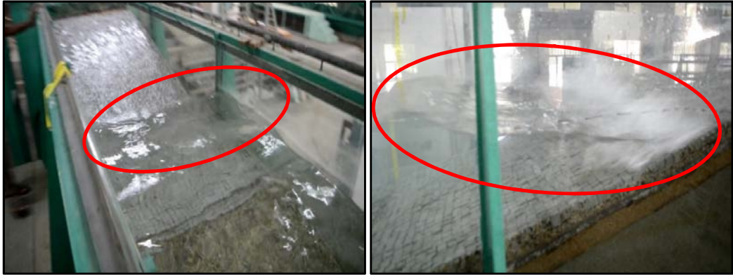
(iv): Wave breaking on revetment
