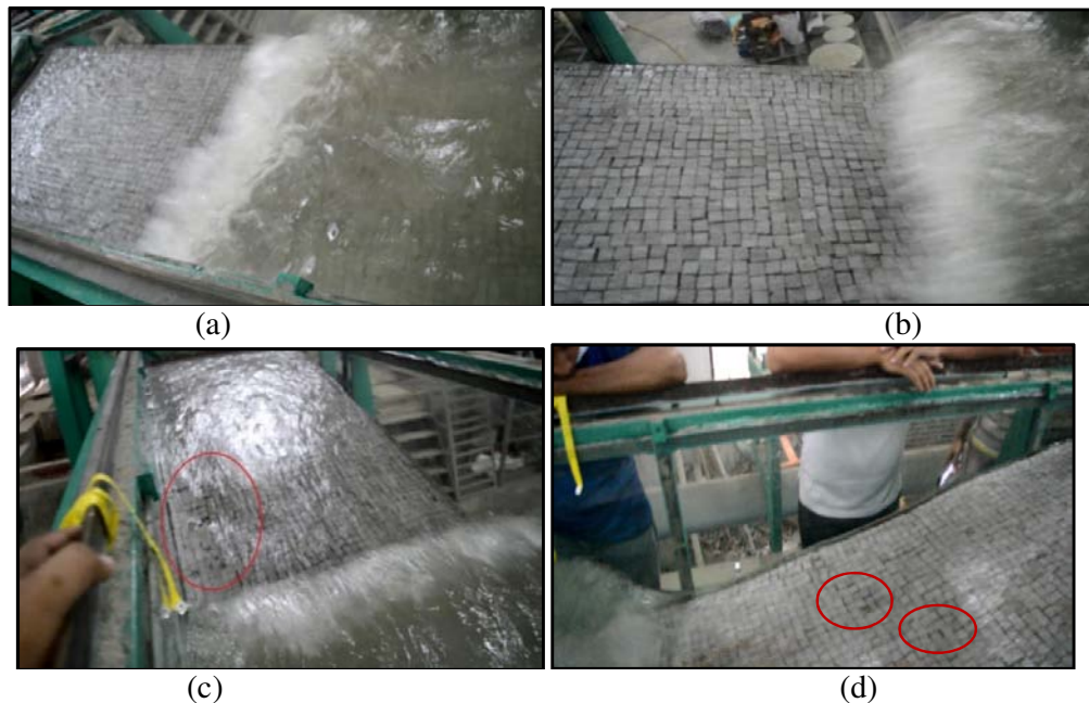
Figure 4.13: Revetment condition for relative breakwater height, h_b/h_w = 0.3
