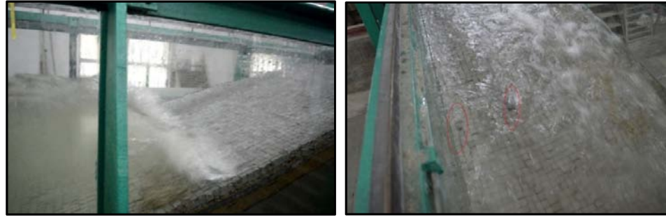
Figure 4.14: Revetment condition for relative breakwater height, h_b/h_w = 0.4
