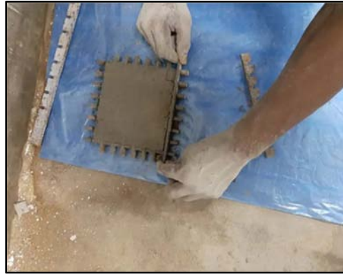
(iv) Removing the formwork
