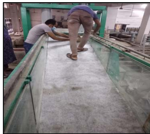
(iv) Placing Geo-textile filter
