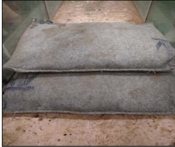
Figure 3.7: Geotextile tube filled with sand
