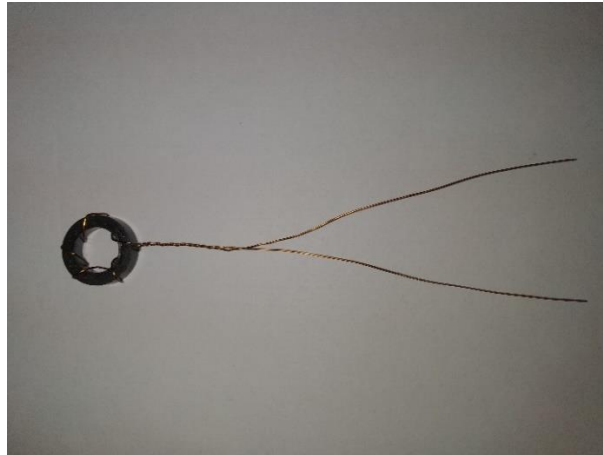
Fig. 3.10 Toroid shaped sample for the measurement of permeability.
