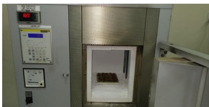
Fig. 3.2 A typical programmable electric furnace inside samples.
