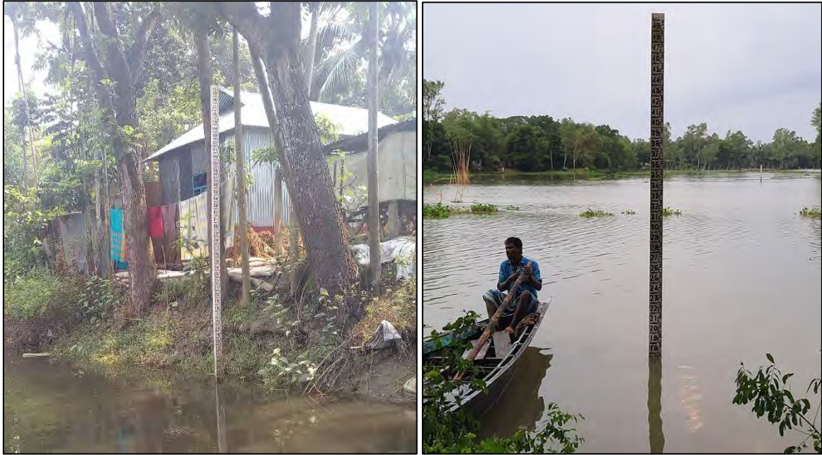
Figure 4.2 Installed Water Level Gauges in the Ranigram Area
