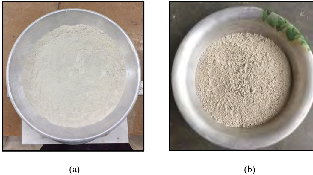
Figure 3.5 Prepared mineral filler samples (a) medical waste incineration fly ash (b) stone dust filler
