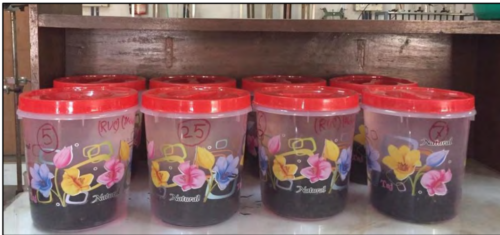
Figure 3.12 An arrangement of the leaching test (according to NEN 7345) being carried out in the laboratory with MWIFA incorporated Marshall samples
