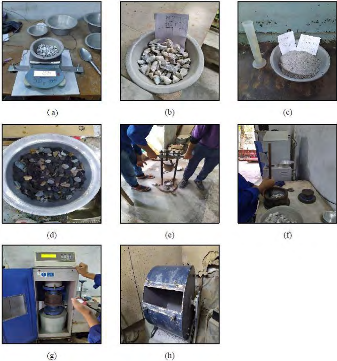
Figure 3.2 (a) Sample measuring for testing (b) Labeling for the certain test (c) Pycnometer for specific gravity test of fine aggregates (d) Coarse aggregates were soaked for achieving SSD condition (e) Aggregate impact value test (f) Tamping with rod in different layers (g) Compression testing machine for ACV, TFV tests (h) Los Angeles Abrasion test
