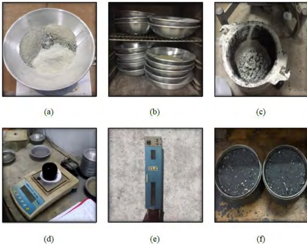
Figure 3.8 Specimen preparation steps: (a) Weighing batch mix (b) Heating in oven (c) Batch mix in mechanical mixer (d) Bitumen measuring (e) Compaction machine (f) Compacted mould
