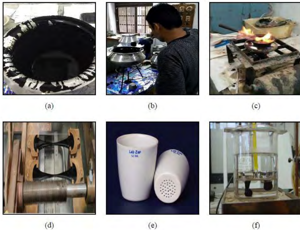
Figure 3.3 (a) Raw bitumen (b) Bitumen heated in burner before testing (c) Flash and fire point testing (d) Ductility testing of bitumen (e) Gooch crucible for solubility testing (f) Ring and Ball apparatus for softening point determination
