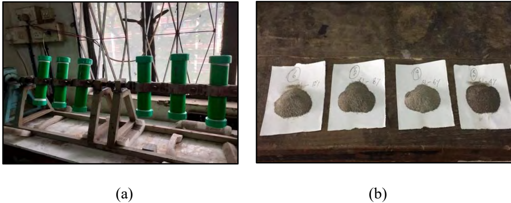
Figure 3.11 a) TCLP test setup (b) Powdered samples from moulded specimens
