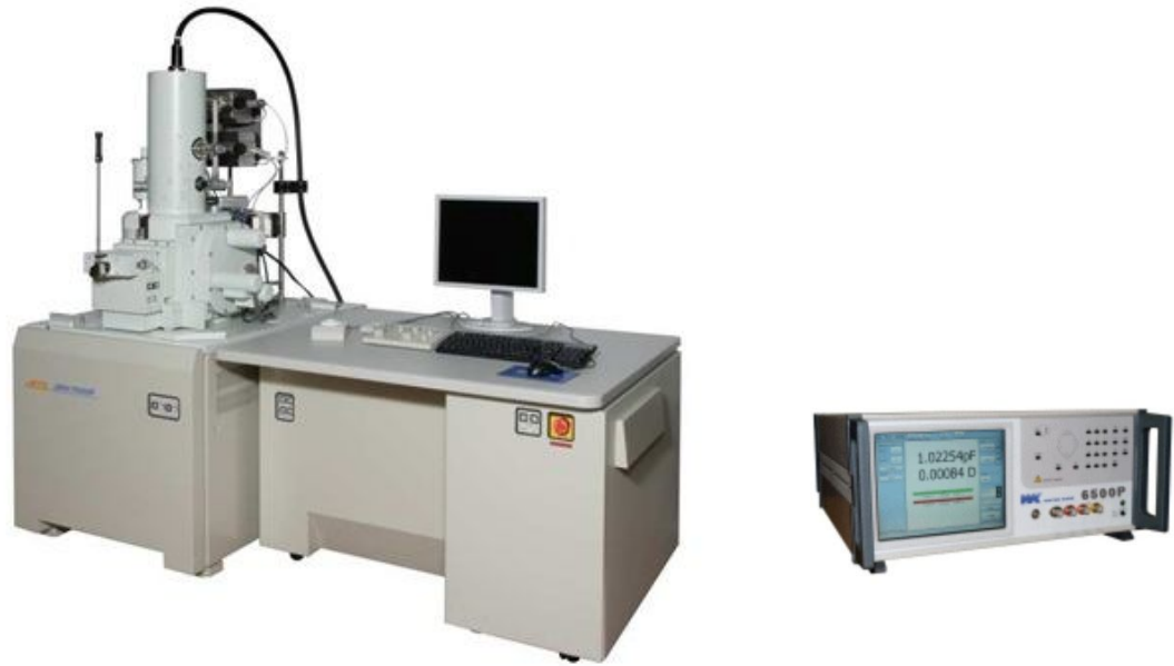
Fig. 3.3: Experimental setup for characterization and dielectric property measurement (a) FE-SEM for microstructural analysis, (b) Impedance analyzer for dielectric property measurement
