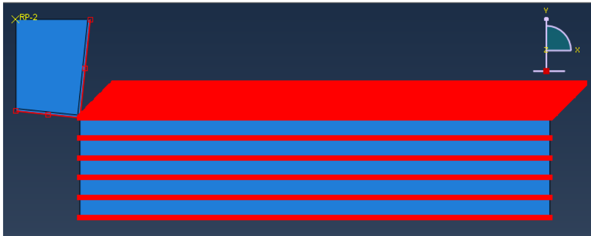
(a) Surface to surface contact
