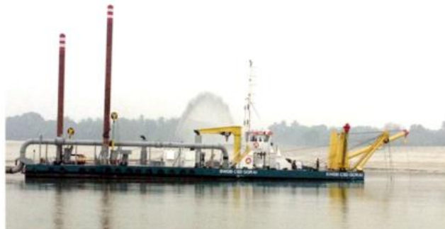
Figure 2-7: Maintenance dredging of the main River System as routine activities of BIWTA for maintaining the river navigability at critical location (Source: Google)
