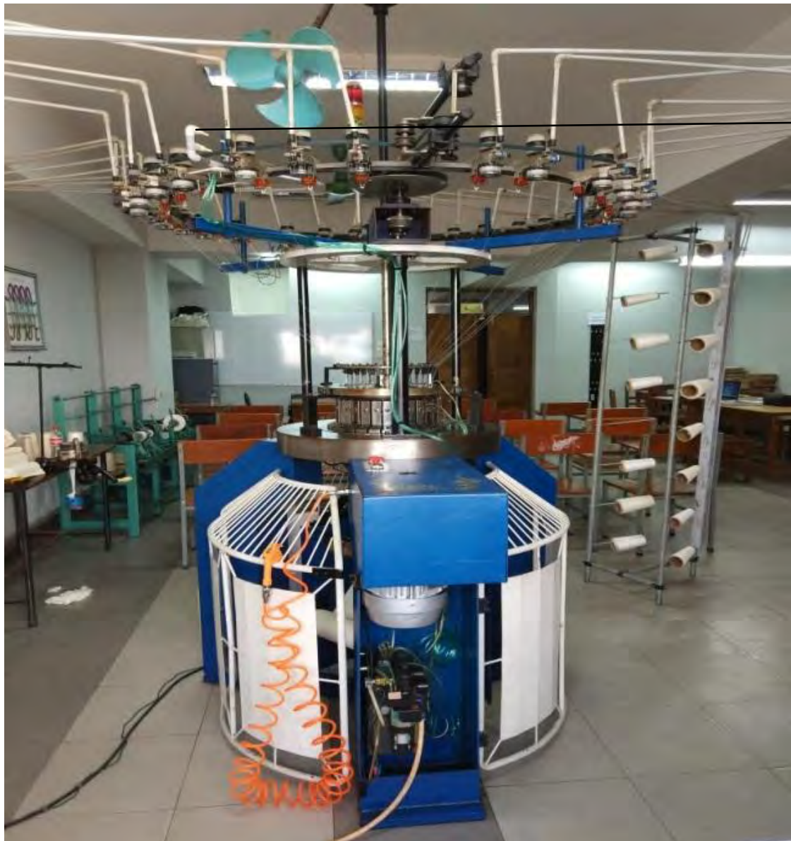
Figure 7.52: The newly developed lint removal device attached to a knitting machine
