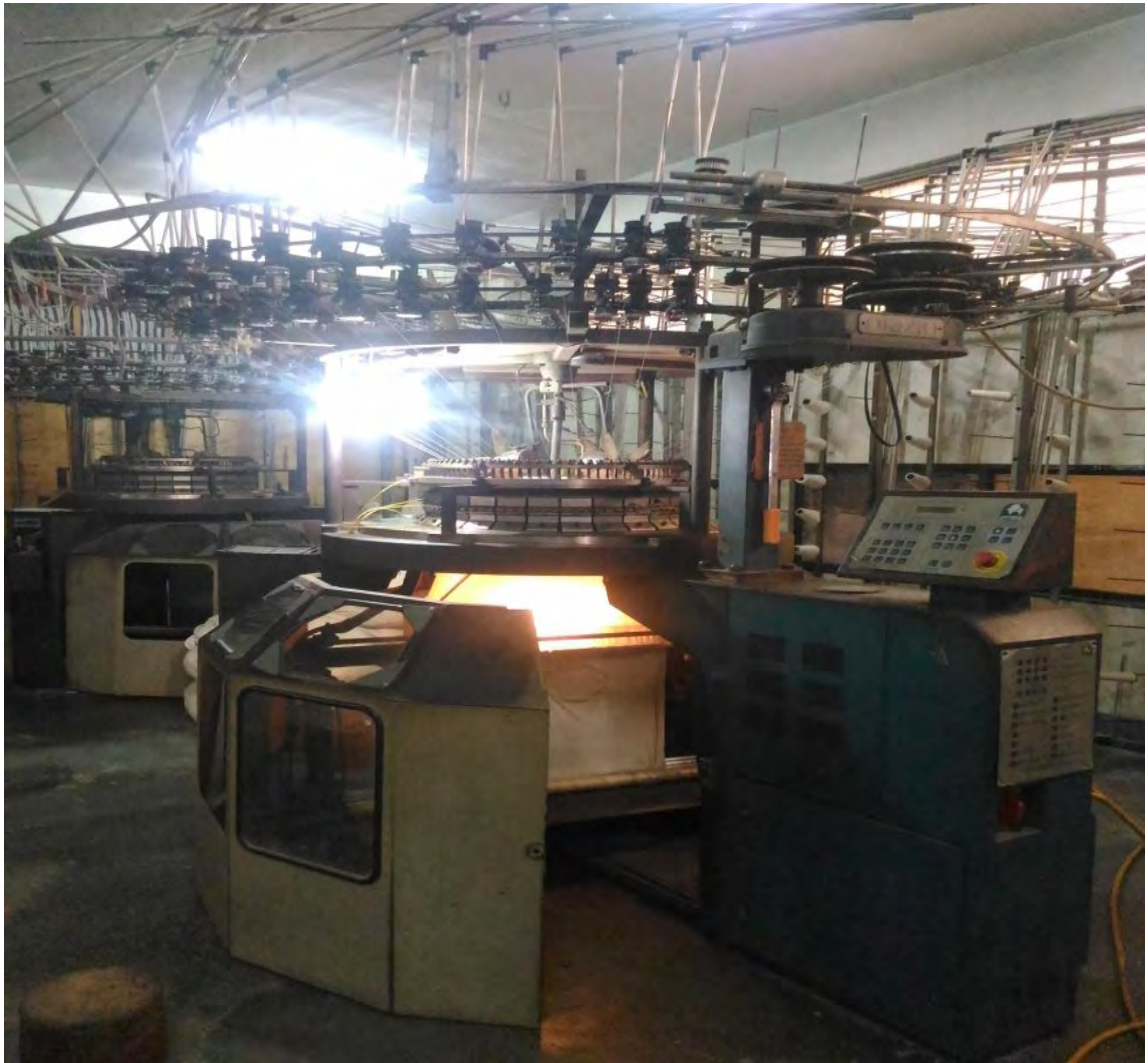
Figure 1.3: A circular weft knitting machine (Courtesy: Padma Polycotton Knit Fabrics Limited)
