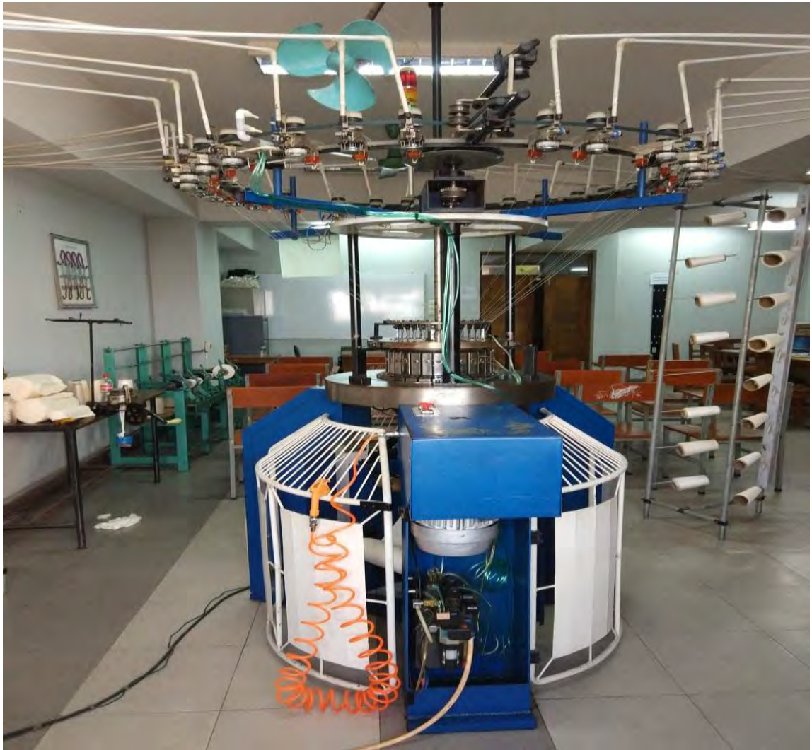
Figure 1.5: Single jersey circular knitting machine ( Courtesy: Knitting laboratory, Department of Textile Engineering, Ahsanullah University of Science and Technology )
