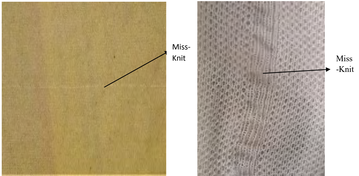
Figure 7.21: „Miss-Knit“ in knitted fabrics; Left - Due to single yarn missing from a double yarn course Right- Due to wrong design in some area of fabric
