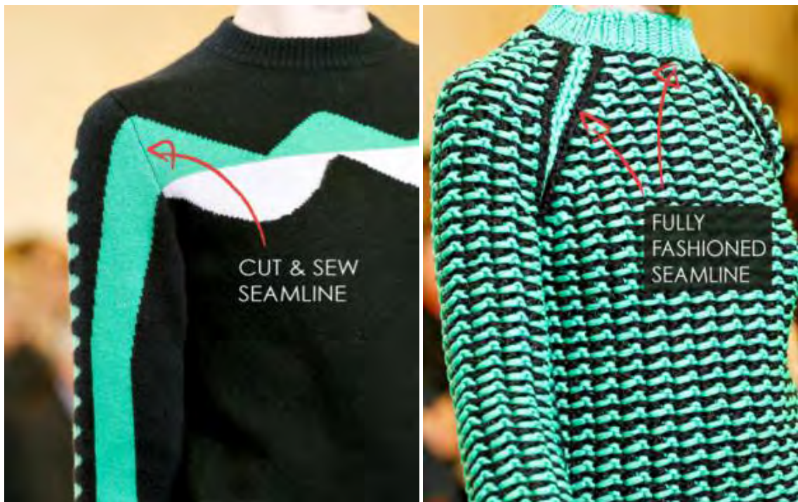
Figure 3.2: Differences between „Cut and sew“ knitwear and „Fully fashioned“ knitwear (Fully Fashioned and Cut and Sew Knitwear at Jil Sander, „n.d.“) (Top: Garment panels for „cut and sew“ knitwear and fully fashioned knitwear; Bottom left: Seam line in a „Cut and sew“ knitwear; Bottom right: Fully-fashioned seamline in a „Fully-fashioned“ knitwear)
