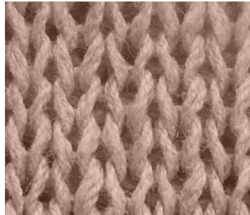
Figure 1.2: Interlooping in knitted fabric
