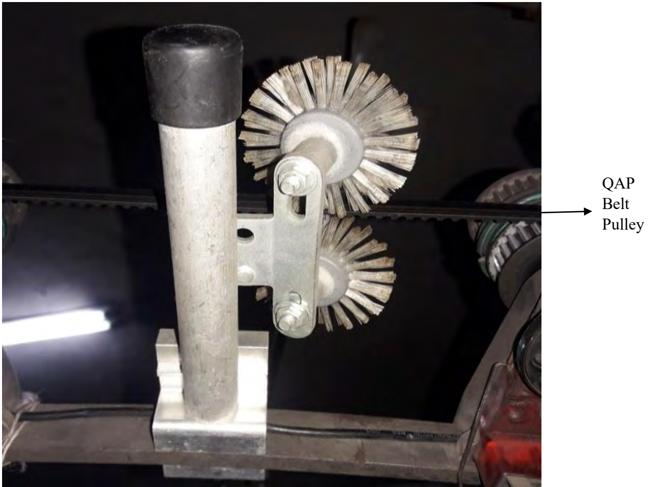
Figure 7.47: An image of single brush-shelf based belt cleaning brush (Courtesy: Padma Polycotton Knit Fabrics Ltd.)
