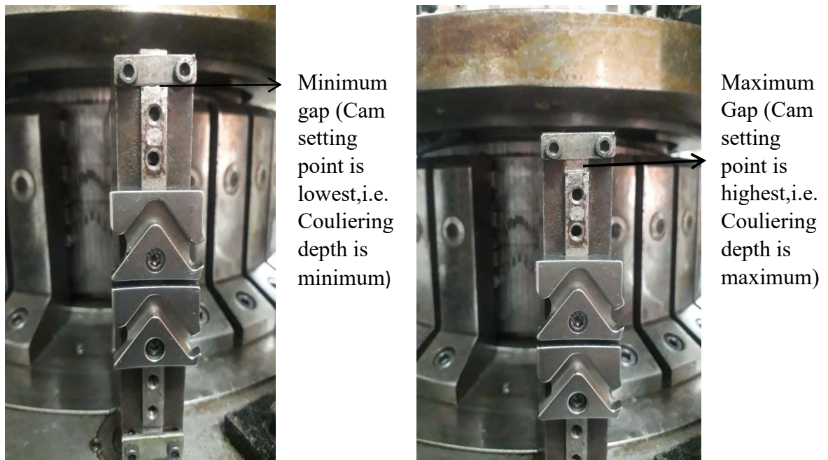
Figure 3.31: Couliering through vertical shifting of cam (Left-Minimum, Right-Maximum)
