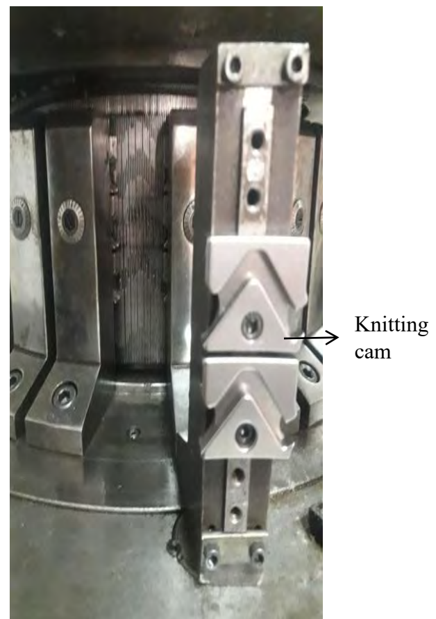
Figure 3.30: Inside view of a cambox
