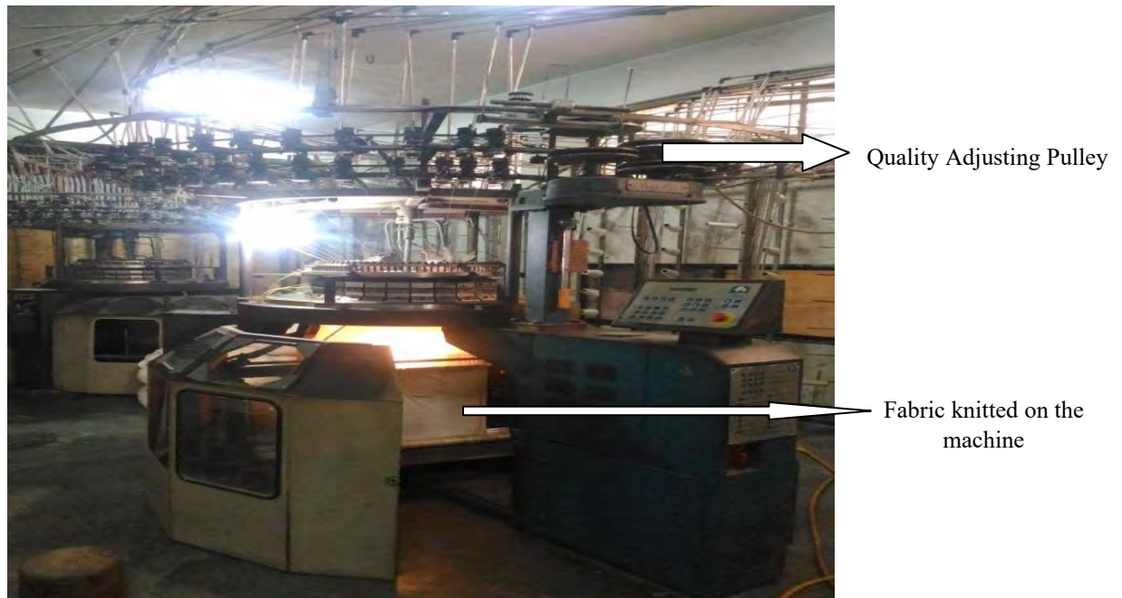
Figure 4.10: The experimental circular knitting machine (Orizio, Johnan) at Padma Polycotton Knit Fabrics Limited
