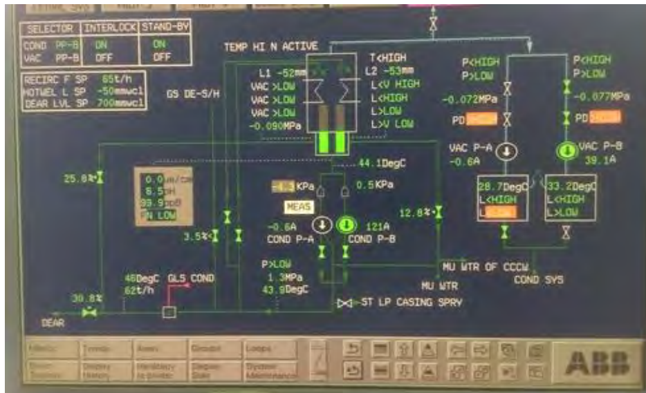
Figure 1: Condensate Pump Flow system.
