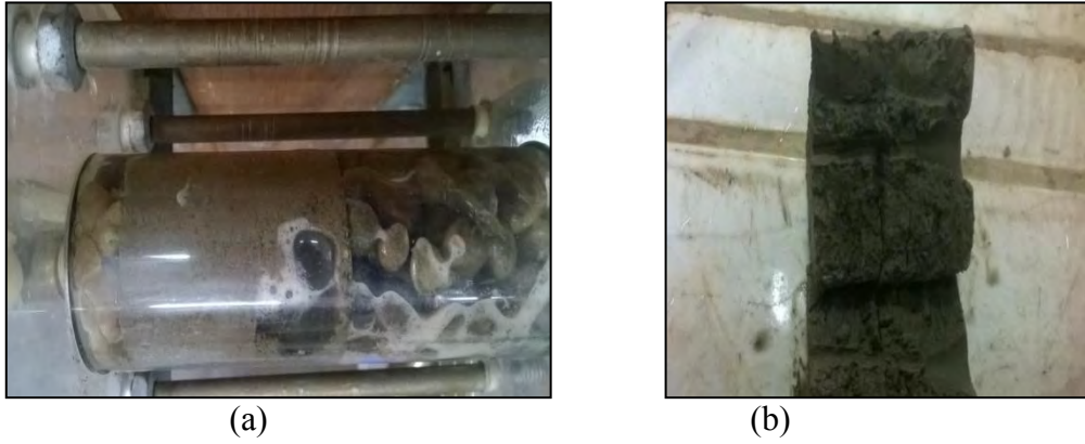
Figure 4.6: Pinhole test for Sample 2: (a) eroded soil inside the tube of pinhole apparatus at 180 mm head, (b) diameter of soil could not be measured as soil eroded from side
