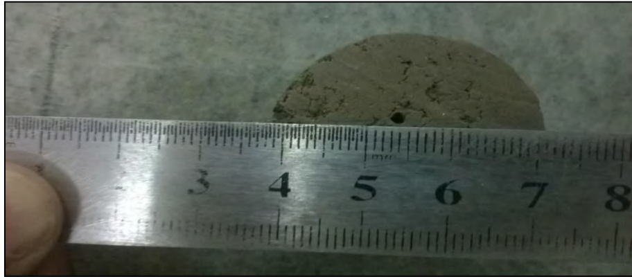
Figure 4.14: Condition of soil sample prepared with 6% fly ash after pinhole test (final diameter of the hole is about 1.2 mm)
