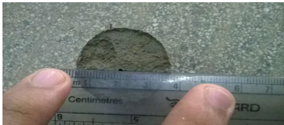
Figure 4.15: Condition of soil sample prepared with 9% fly ash after pinhole test (final diameter of the hole is about 1.00 mm)
