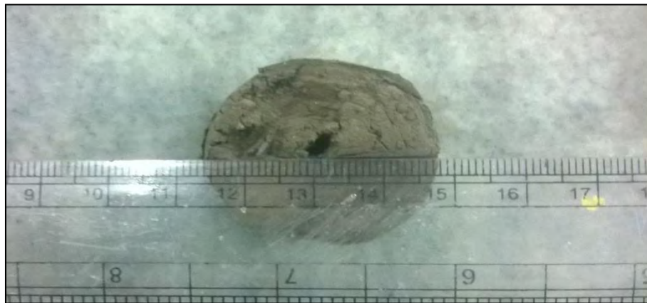
Figure 4.13: Condition of soil sample prepared with 3% fly ash after pinhole test (final diameter of the hole is about 2 mm)
