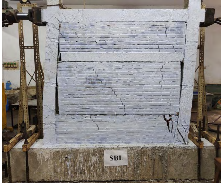
Figure 4.10: SBL at complete failure (at cycle 4).
