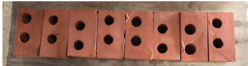
Figure 3.13: Eight half-scale bricks produced from a single full-scale brick.
