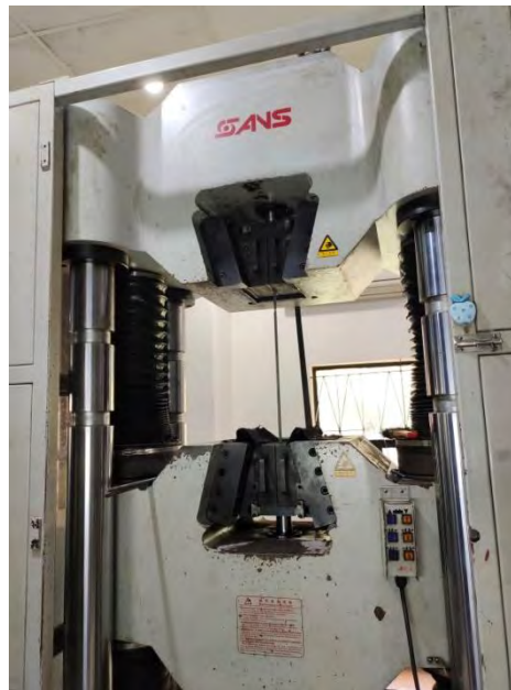
Figure A.1: Testing of rebar.
