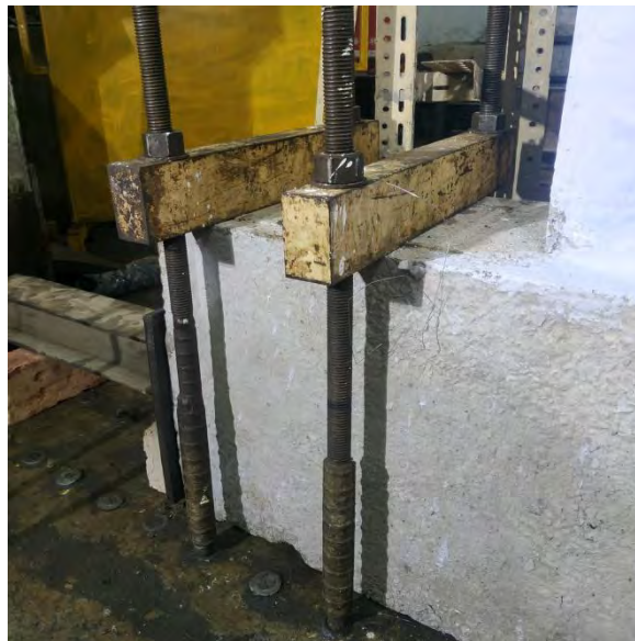
Figure 3.18: Anchor bolt and steel plate.
