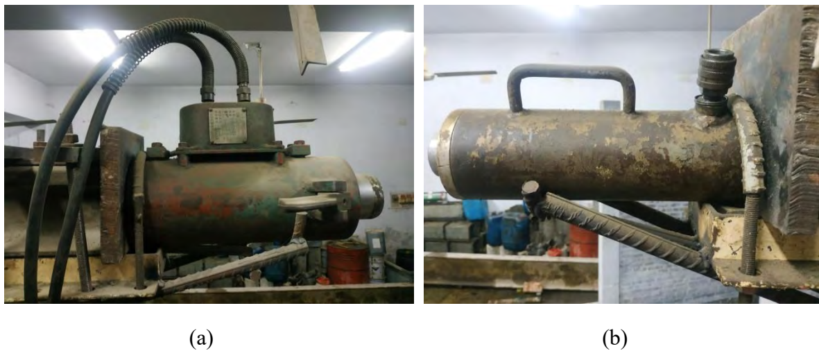
Figure 3.21: (a) Hydraulic Jack 1, (b) hydraulic jack 2.
