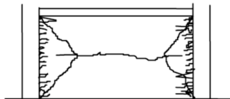
Figure 2.14: Typical degree of damage for bed joint sliding (FEMA 306, 1998).
