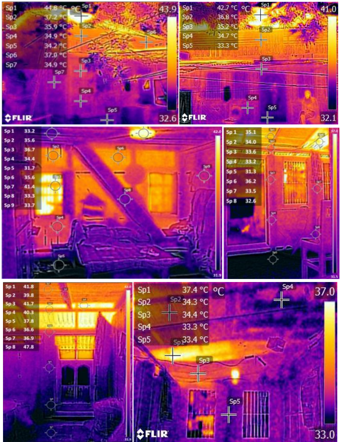
Figure 4.37 Indoor and outdoor surface temperature of a traditional double-storied timber house (Top: outdoor; Middle: ground floor front and middle room; bottom: indoor: first floor)
