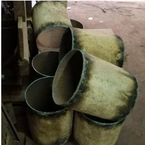
(a) MS pipes before welding of plates
