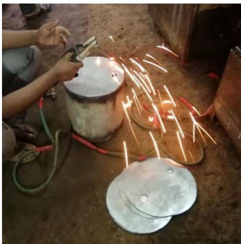
(c) Welding of rear MS plate
