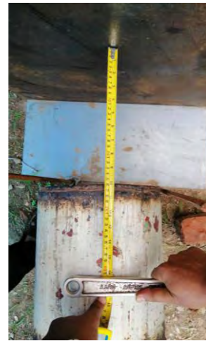
(b) Measuring standoff distance
