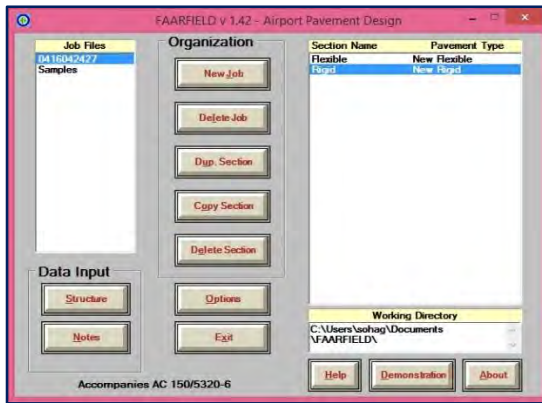
Figure 3.7: FAARFIELD windows for rigid pavement startup.
