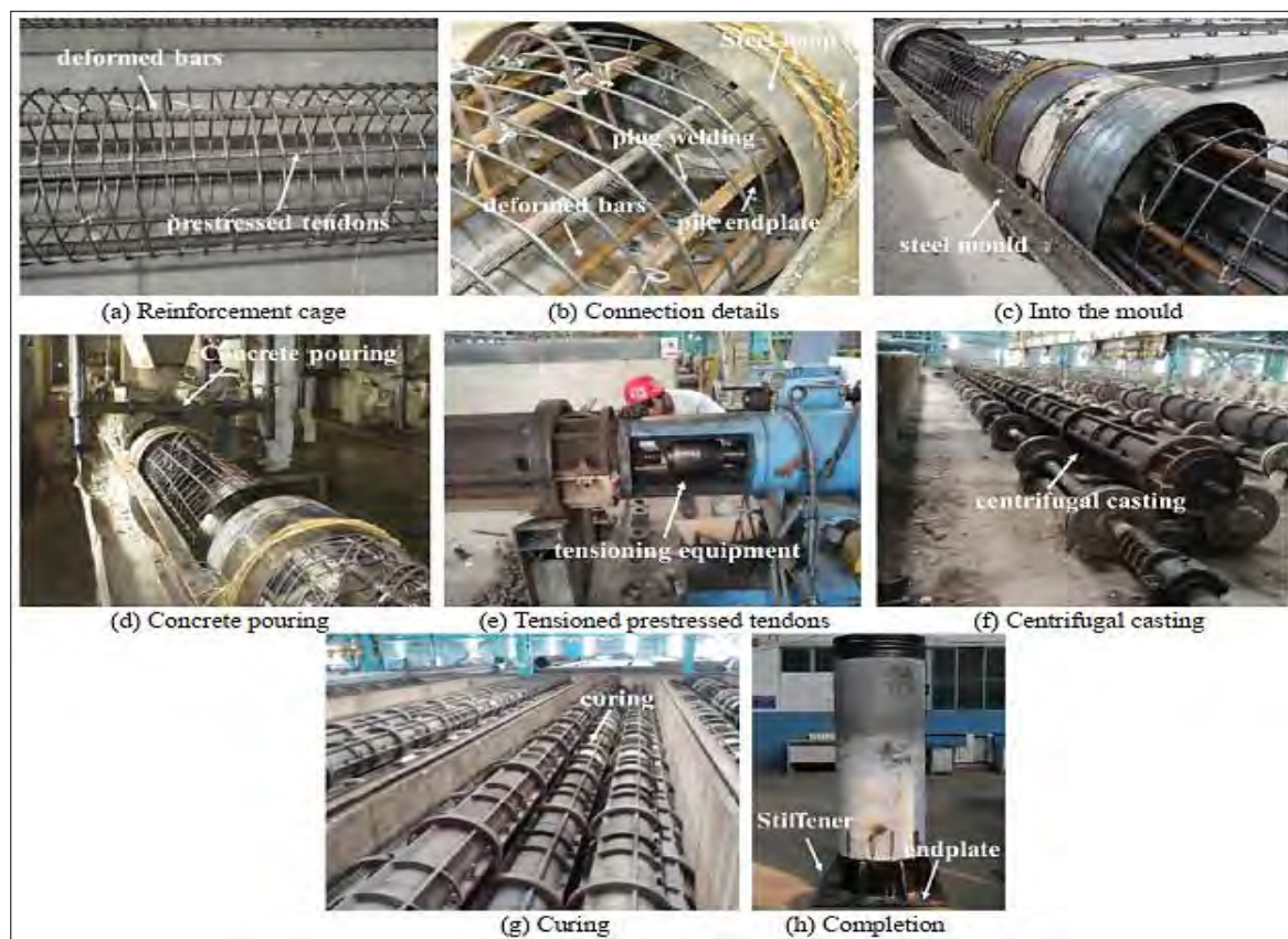
Figure 2.6: Prefabrication process of prestressed piles: (a) Reinforcement cage (b) Connection details (c) Into the mold (d) Concrete pouring (e) Tensioned prestressed tendons (f) Centrifugal casting (g) Curing (h) Completion, (After Xizhi et al., 2020)
