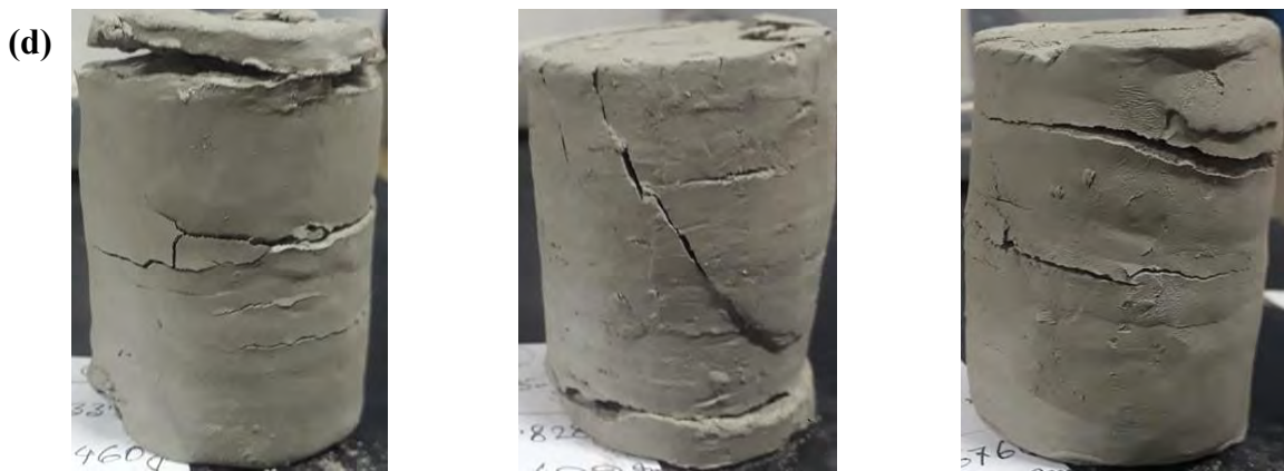
Figure 3.11: Relationship between (a) Shear stress and principal stress (b) Deviator stress and axial strain (c) Volumetric strain and axial strain and (d) shear failure modes of soil samples
