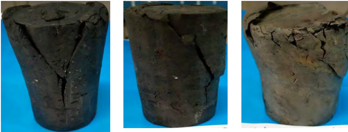
Figure 3.9: (a) Relationship between axial strain and stress and (b) brittle failure mode
