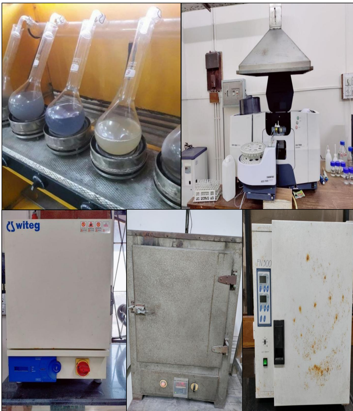
Figure 3.10: Lab facilities used to dry and ash leather sample, determine chromium and extract gelatin
