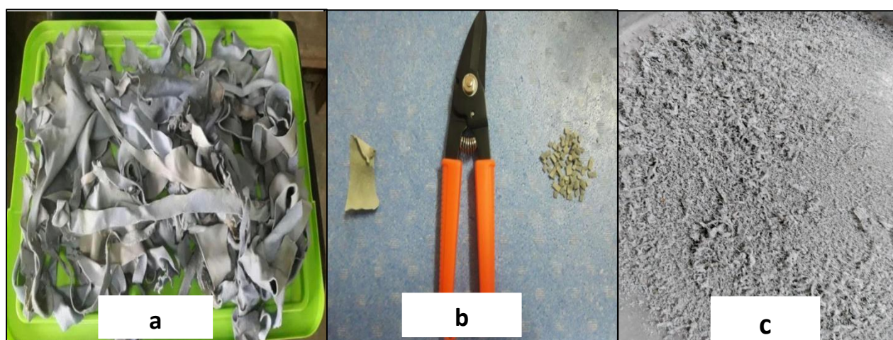
Figure 3.1: a) chrome-tanned trimmings b) leather cutting tool c) chrome-tanned shavings
