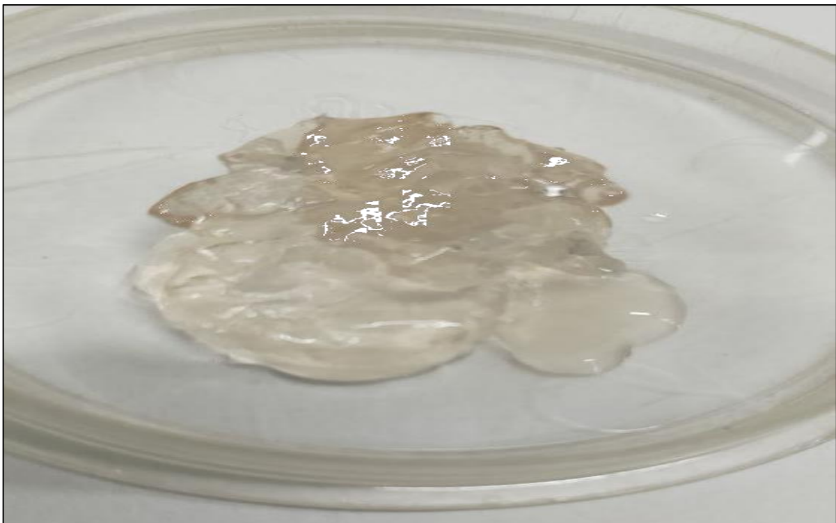
Figure 3.13: aqueous gelatin from dechromed shavings (2hrs extraction)
