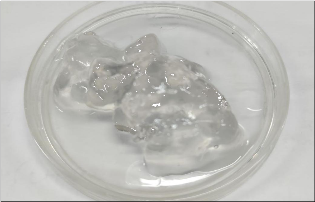
Figure 3.12: Aqueous gelatin from dechromed trimmings (1hr extraction)
