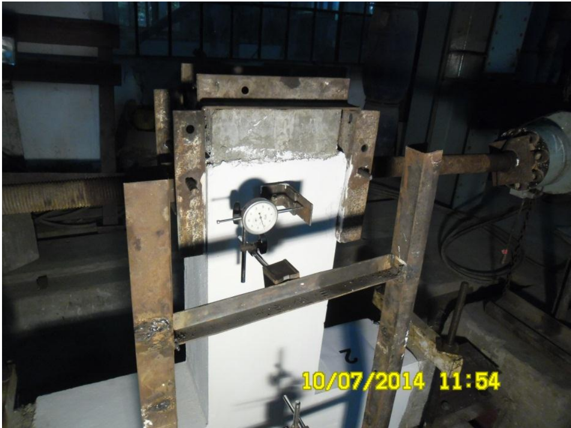
Fig.3.15: Dial gauge set up
