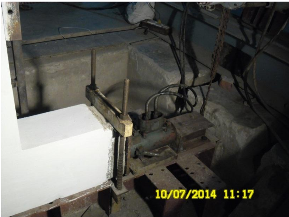
Fig.3.13: Column axial load arrangement by hydraulic jack
