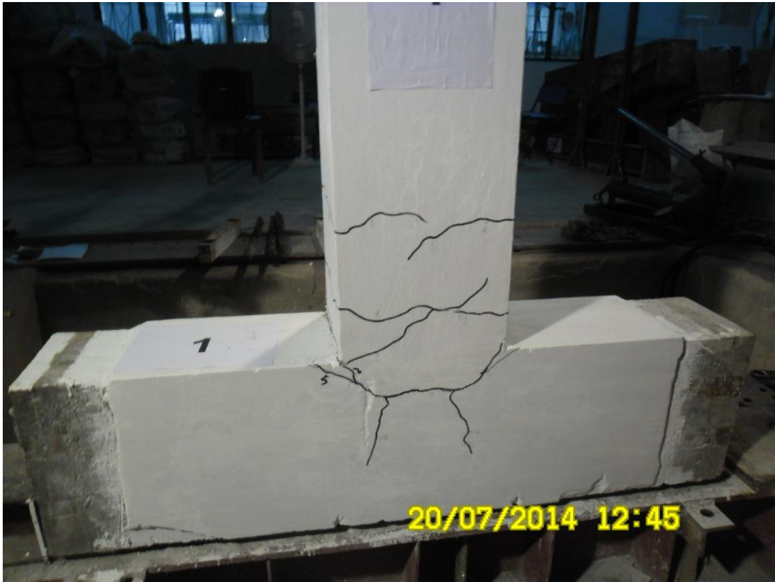
Fig.4.2: Cracking type of failure in reference specimen RS1
