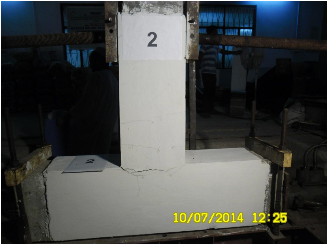
Fig.4.6: Cracking type of failure in ferrocement jacketed specimen JS1
