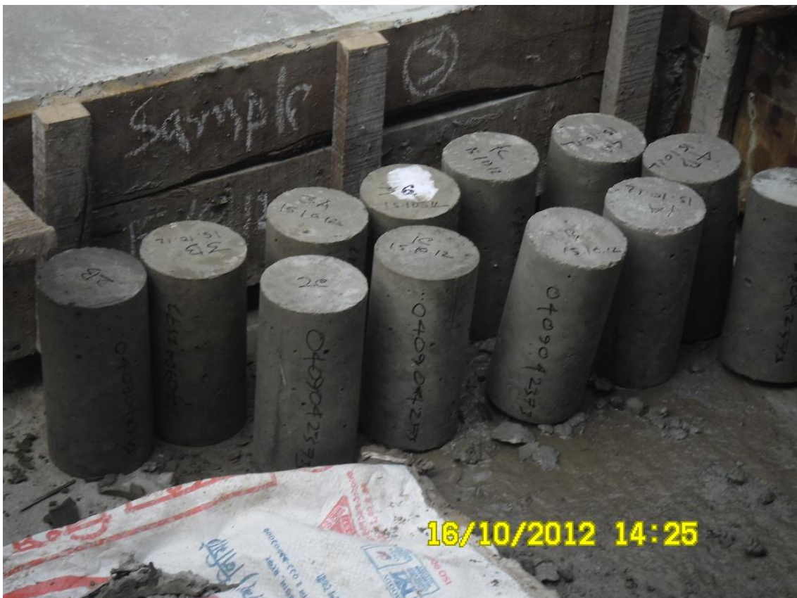
Fig.3.10: Concrete cylinders for compressive strength test
