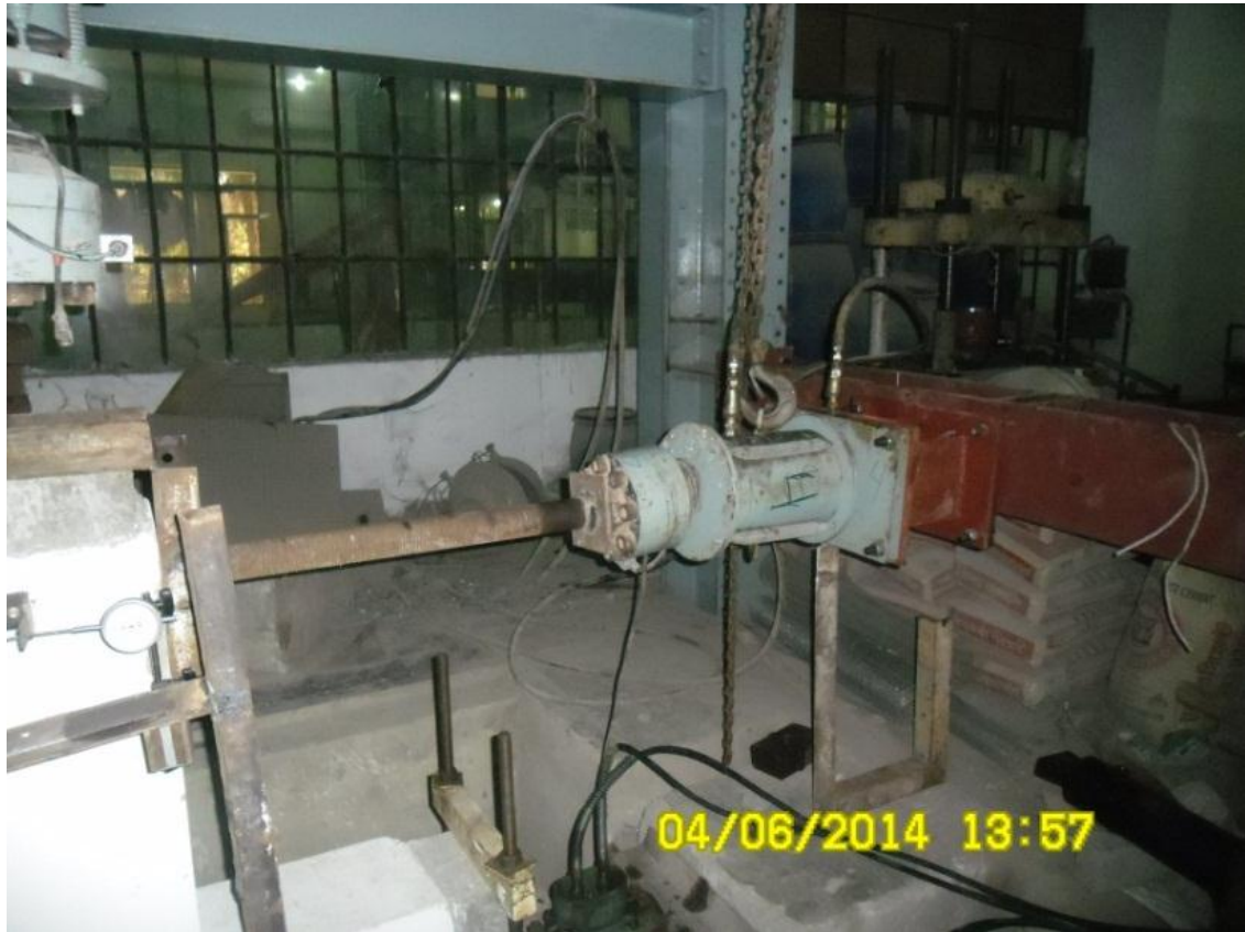
Fig.3.14: Beam lateral loading arrangement
