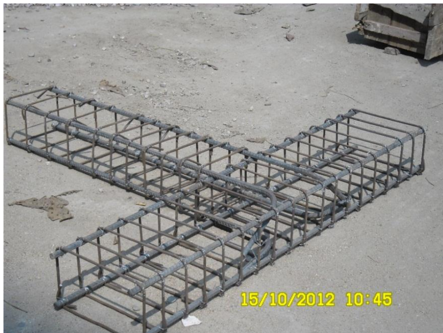
Fig.3.4: Fabricated reinforcement for test specimen
