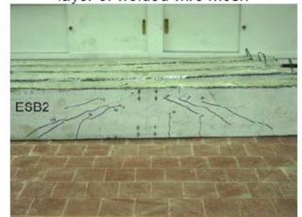
Group 7: Light brick core and single layer of expanded wire mesh
