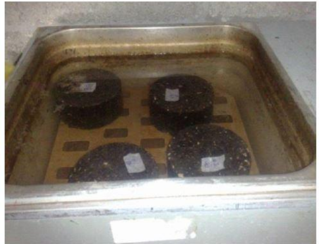
Figure P.7: Water bath for Marshal Samples
