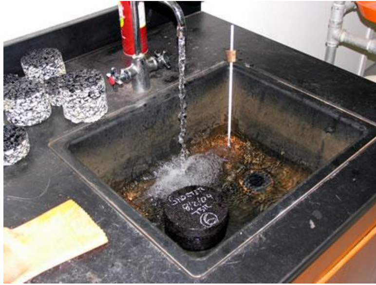
Figure 2.23: Filling the 2-hour room temperature water bath.
