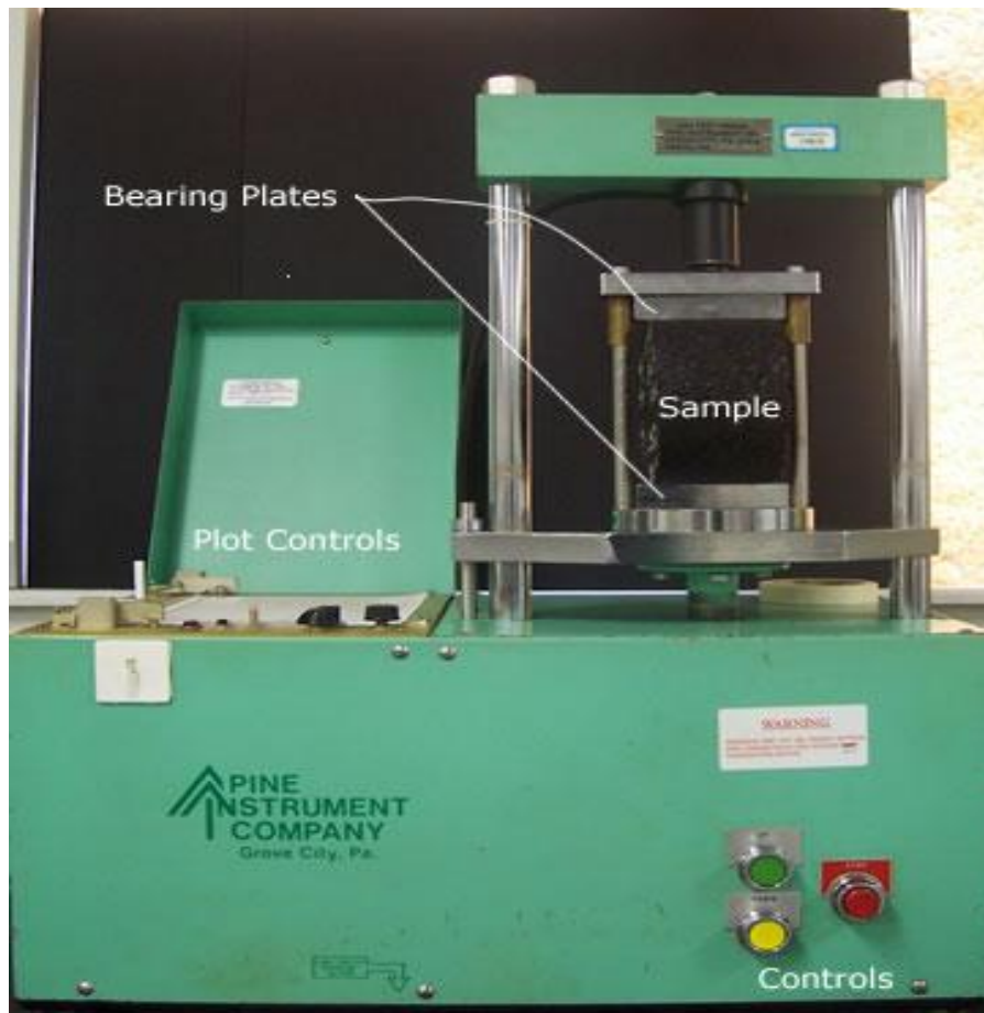
Figure 2.20: Split tensile test setup.
