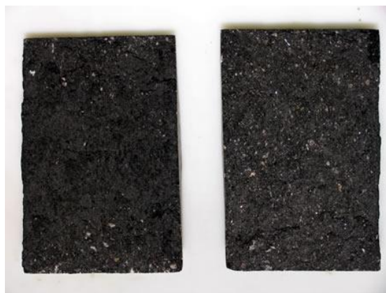
Figure 2.16: HMA samples with no moisture damage (left) and moisture damage (right). A more subtle example than Figure 2.15 , but still with noticeable uncoated aggregate.
