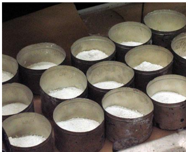
Figure 2.19: Lime in small containers for addition during mix design sample preparation.
