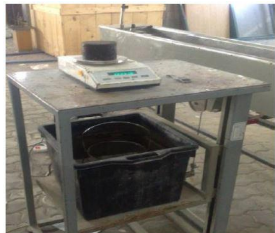
Figure P.5: Marshal Samples weighting in water
