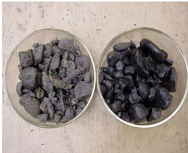
Figure 2.18: Aggregate on left has severe stripping. Right has 0.5 percent by weight asphalt binder antistripping modifier.
