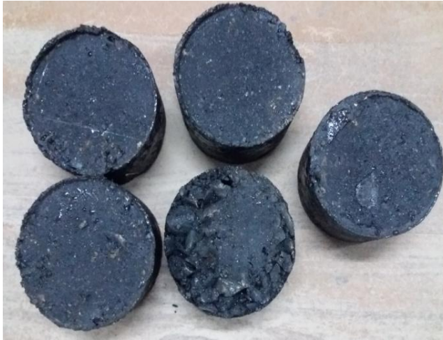
Figure P.6: Cement mixed Marshal Samples
