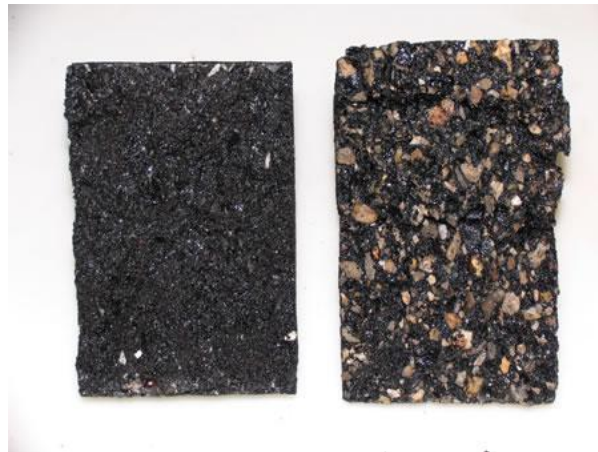
Figure 2.15: HMA samples with no moisture damage (left) and moisture damage (right). Notice the amount of uncoated aggregate on the damaged sample.
