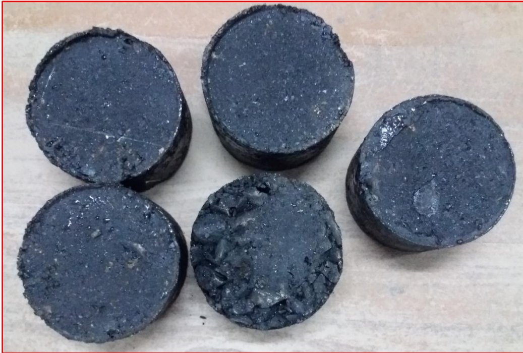
Figure 3.7: Marshall Specimens with cement as filler material
