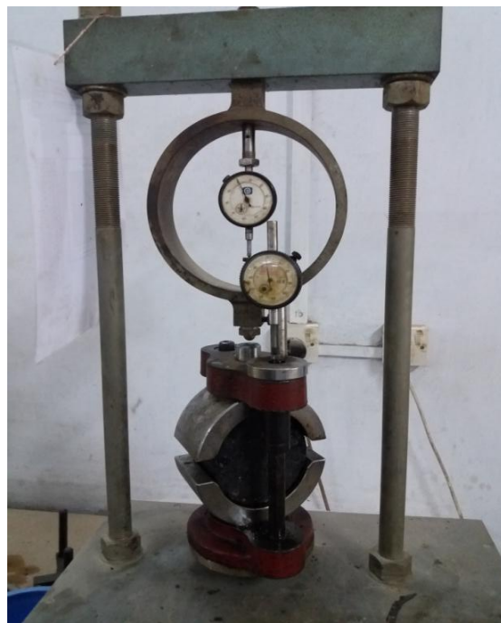
Figure P.8: Testing Marshal Samples for stability and flow
