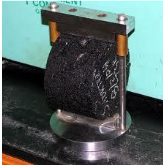
Figure 3.9: Sample placed between the bearing plates before testing
