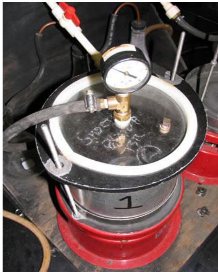
Figure 2.21: Vacuum saturation of a sample ( https://pavementinteractive.org/reference-desk/testing/asphalt-tests/moisture-susceptibility/ )
