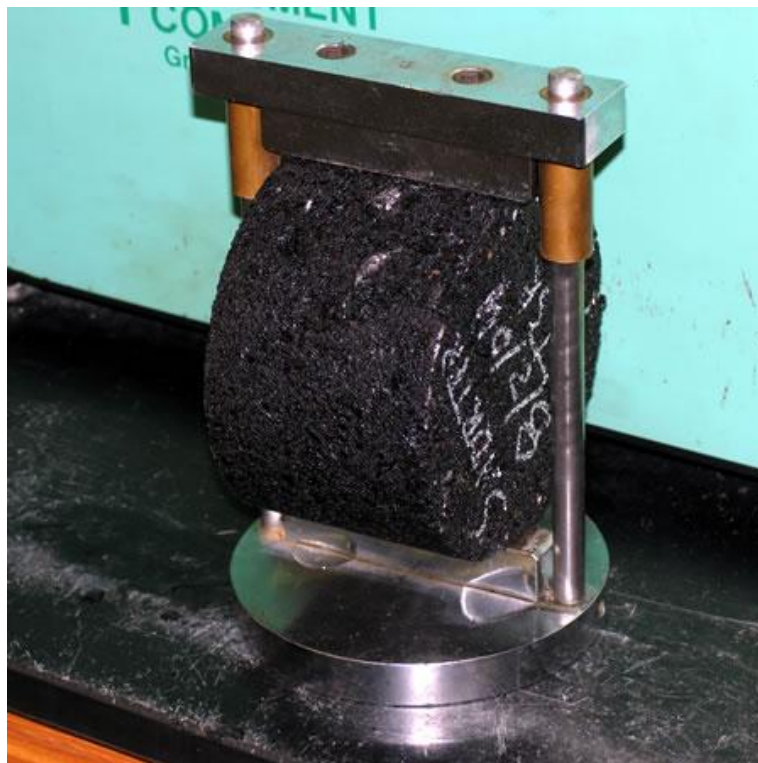
Figure 2.24: Sample placed between the bearing plates before testing.
