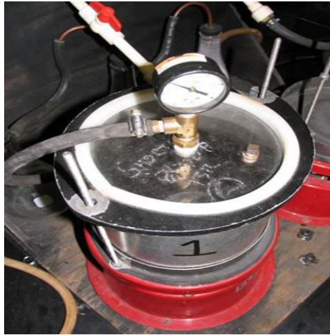
Figure 3.8: Vacuum saturation of a sample.
