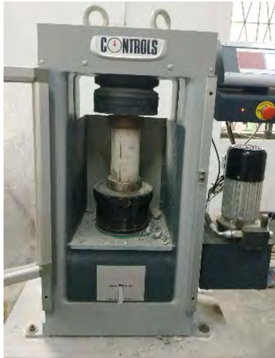
Figure 3.1 Compression test set-up
