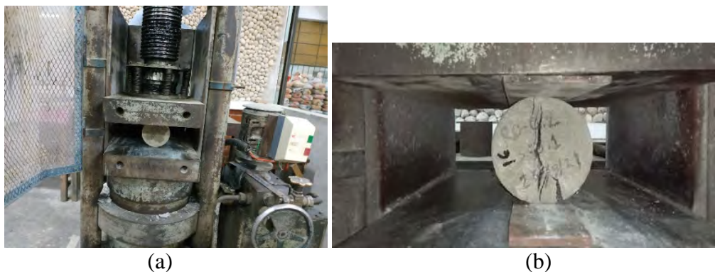
Figure 3.4 Splitting tensile test (a) setup (b) failure pattern of nylon fiber reinforced concrete cylinder
