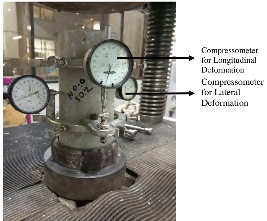
Figure 3.3 Sample fitted within a compressometer
