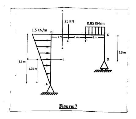
(b) Determine the internal system of forces at section a-a and section b-b.
