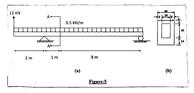
(a) Draw Axial Force, Shear Force, and Bending Moment diagram using the method of section for the beam in the figure below.
