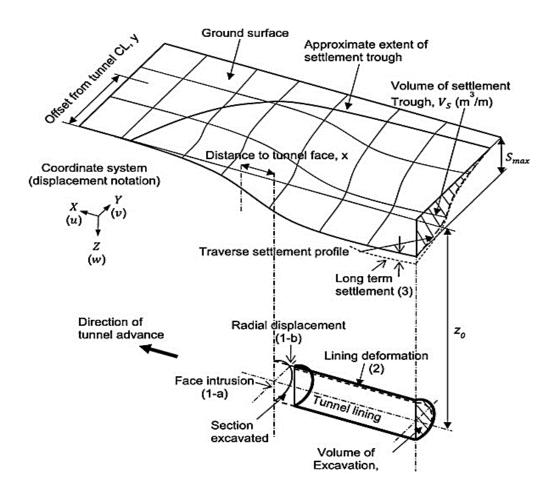
Figure 2.24: Geometry of the tunnel induced settlement trough (Attewell, 1986)
