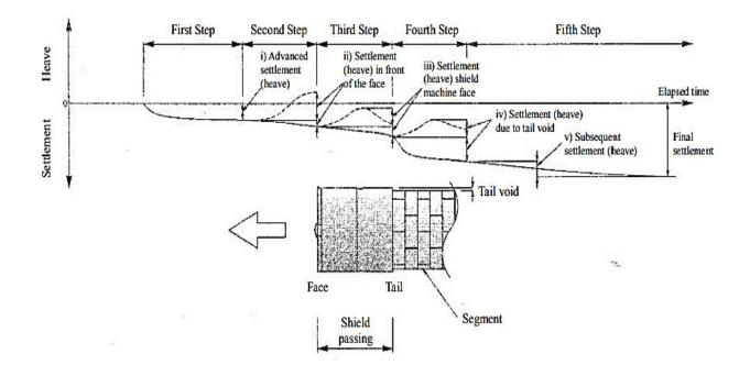
**Figure 2.22:** Classification of ground movement due to shield advancement (Tamagnini et al., 2022)
