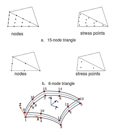
**Figure 2.32:** Topology of 15 node wedge elements, 6 node triangles and 16 node interface elements in PLAXIS 3D (Galavi et al., 2013)
