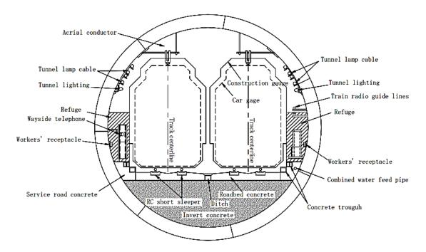
**Figure 2.15:** Example of facilities and structure of a double-track railroad tunnel (TBM) (Harer et al., 2008)
