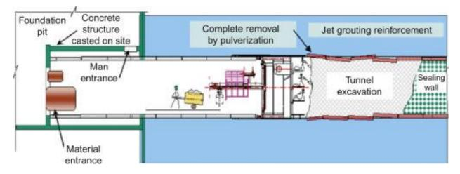
Figure 2.13: Construction Procedure of TBM-EPB Method (Source: Internet)
