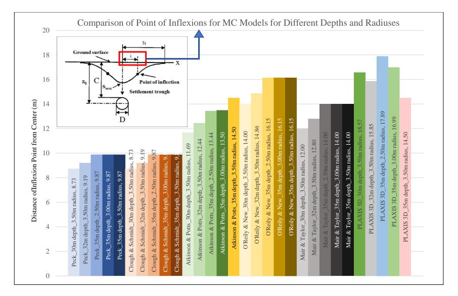
**Figure 4.23:** Comparison of Distance of Inflexion Points for MC Models for Different Depths (30m, 32m, 35m) and Different Radiuses (2.5m, 3m, 3.5m)
