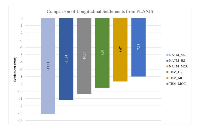
Figure 4.35: Longitudinal Settlements for both NATM and TBM methods considering 35m depth and 3.50m radius (from PLAXIS)
