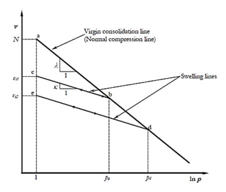
Figure 2.42: Behavior of Soil Sample under Isotropic Compression (Wood, 1990)
