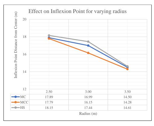
**Figure 4.31:** Effect on Inflexion Point for increasing of radius (2.50m, 3.00m and 3.50m)
