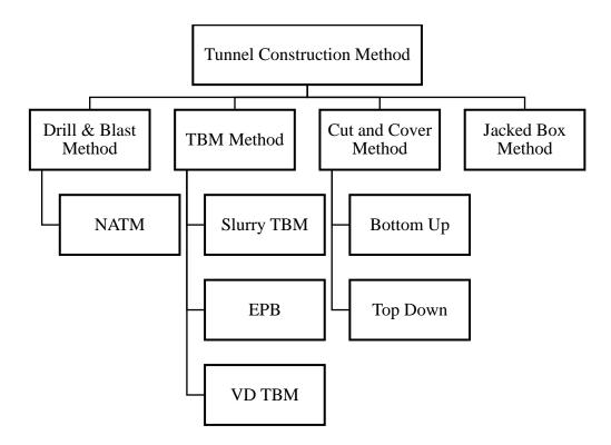
Figure 2.4: Classifications of Tunnel Construction Methods (Tatiya, 2005)
