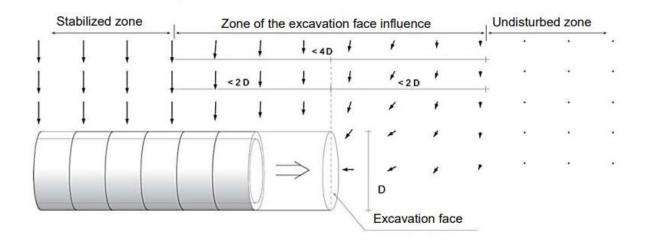
**Figure 2.3:** Influence of the Excavation Face: Ground Mass Displacements (Franca, 2006)
