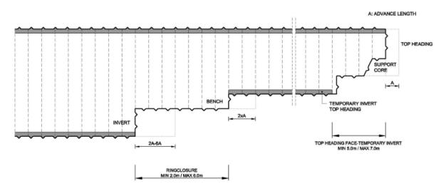
Figure 2.6: Typical Excavation Sequence in Soft Ground Conditions (ICE, 1996)
