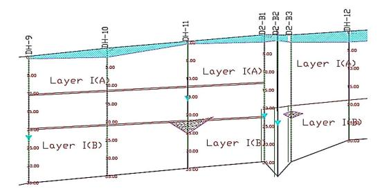
**Figure 3.3:** Geological Section of Mashhad Metro Line 2 (12+500km) (Eslami et al., 2020)
