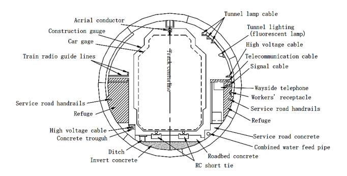
**Figure 2.16:** Example of facilities and structure of a single-track railroad tunnel (TBM) (Harer et al., 2008)
