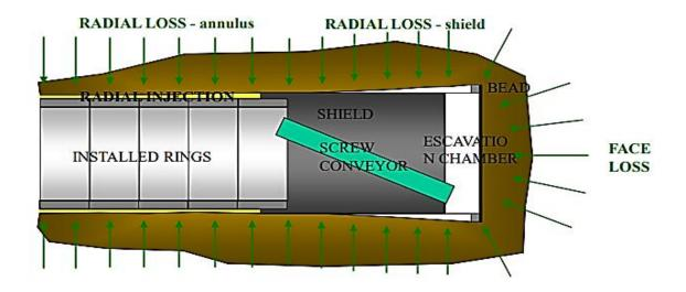
Figure 2.21: Components of the Volume Loss (Golpasand et al., 2016)
