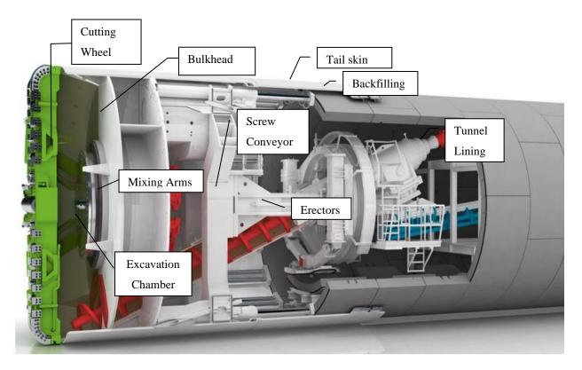
Figure 2.10: Components of a TBM-EPB Machine (Source: Internet)
