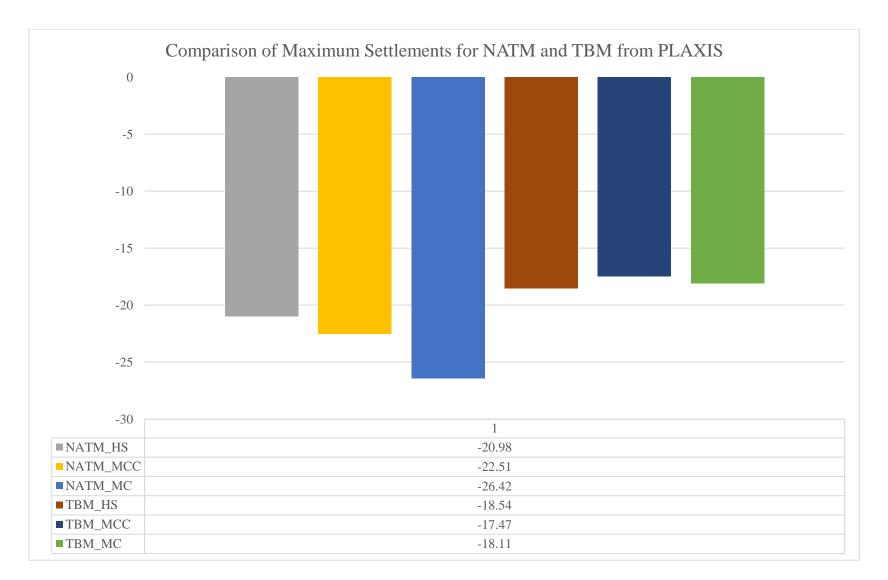
Figure 4.33: Comparison of Maximum Settlement for NATM and TBM Methods from PLAXIS (for different types of models)
