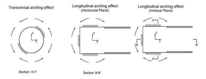
Figure 2.2: Three-dimensional arching effect (Zhao et al., 2007)
