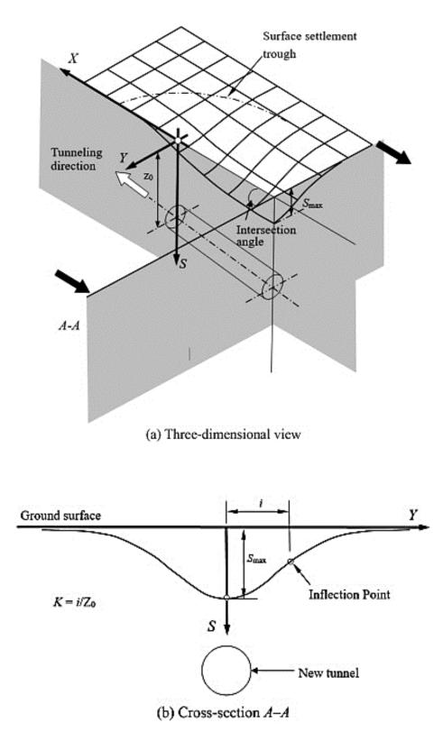
**Figure 3.5:** Distribution of Surface Settlement Trough (a) Three-dimensional view (b) Cross Sectional view (Transverse Section) (Lu et al., 2019)
