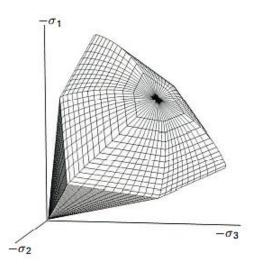
**Figure 2.41:** Representation of total yield contour of the HS model in principal stress space for cohesionless soil (Galavi et al., 2013)
