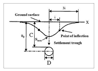
Figure 3.6: Relevant parameters for relations (Eslami et al., 2020)
