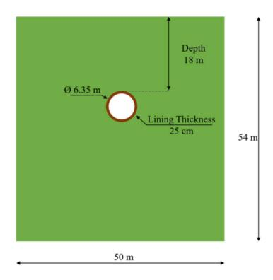
Figure 3.13: Schematic Representation of Model Parameters (Naqvi et al., 2021)
