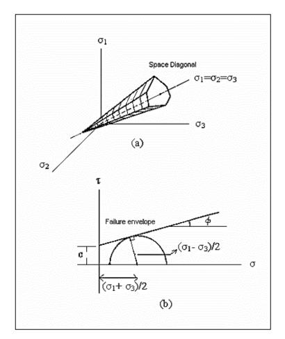
Figure 2.36: Mohr-Coulomb criteria in principal stress space and Mohr's diagram. a) Principal stress space, b) Mohr's diagram (Bentley, 2018)
