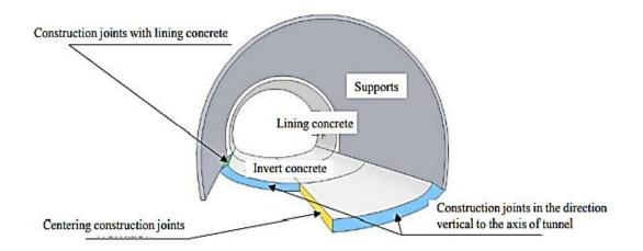
Figure 2.20: Example of Construction Joints in Invert Concrete (Source: Internet)
