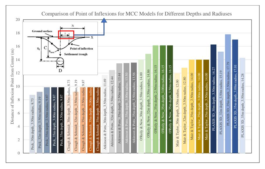
**Figure 4.24:** Comparison of Distance of Inflexion Points for MCC Models for Different Depths (30m, 32m, 35m) and Different Radiuses (2.5m, 3m, 3.5m)
