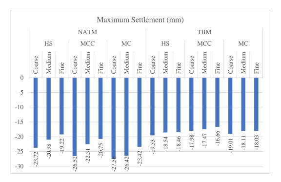
Figure 4.21: Effect on Maximum Settlement due to Refinements of Meshing for Different Models
