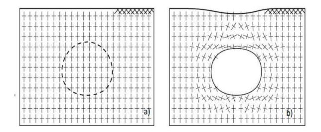
**Figure 2.1:** Direction of the Principal Stresses: a) in an intact soil mass, b) after tunnel excavation (Franca, 2006)
