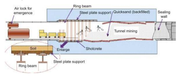
Figure 2.8: Construction Procedure of NATM Method (Schubert, 2001)
