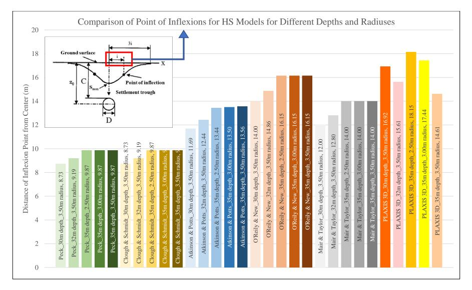
**Figure 4.25:** Comparison of Distance of Inflexion Points for HS Models for Different Depths (30m, 32m, 35m) and Different Radiuses (2.5m, 3m, 3.5m)
