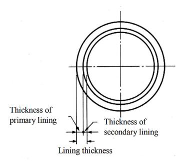
Figure 2.18: Position of Primary and Secondary Linings (Source: Internet)
