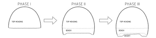
Figure 4.12: Phases of construction used for PLAXIS 3D modelling (Sinha, 1989)
