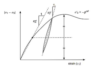
**Figure 2.40:** Definition of  $E_{50}^{ref}$  and  $E_{ur}^{ref}$  for drained triaxial test results (Galavi et al., 2013)
