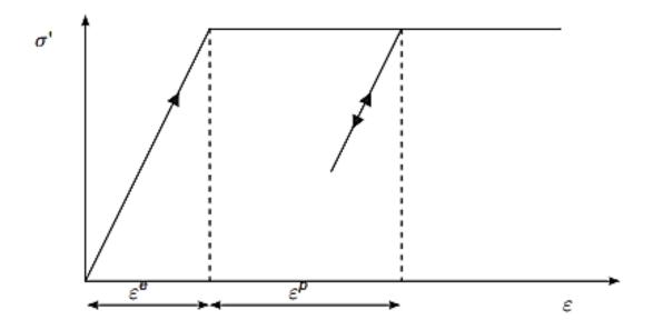
Figure 2.34: Basic Idea of an Elastic Perfectly Plastic Model (Bentley, 2018)
