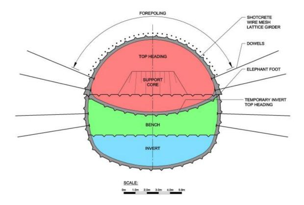
Figure 2.5: Typical Excavation and Support in Soft Ground Conditions (ICE, 1996)
