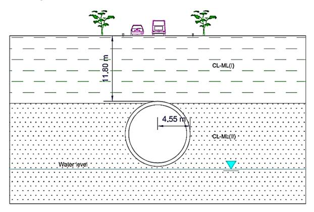
Figure 3.2: Section of ground line 2 Metro of Mashhad (Eslami et al., 2020)
