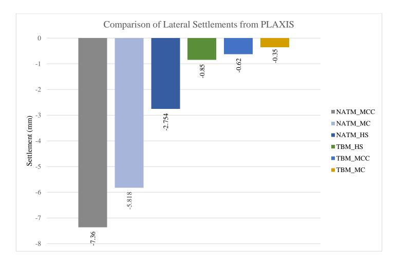
Figure 4.36: Lateral Settlements for both NATM and TBM methods considering 35m depth and 3.50m radius (from PLAXIS)
