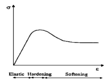
Figure 2.31: Real Soil Behavior involving hardening and softening (Potts, 2001)
