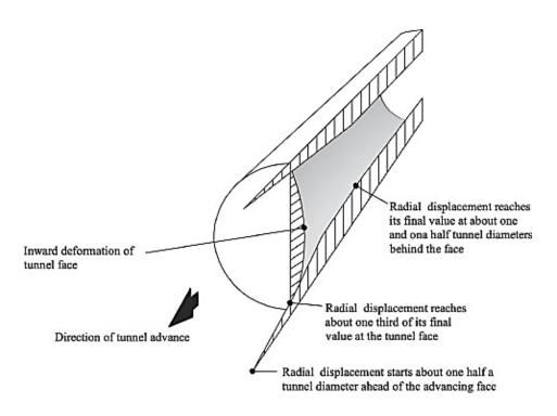
Figure 2.28: Longitudinal Deformation Profile (Luo et al., 2018)
