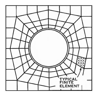
Figure 2.29: Typical Finite Element Model Formation for Tunnel (Luo et al., 2018)
