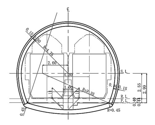
**Figure 2.14:** Example of standard cross section of railway tunnel (NATM) (Daraei and Zare, 2019)
