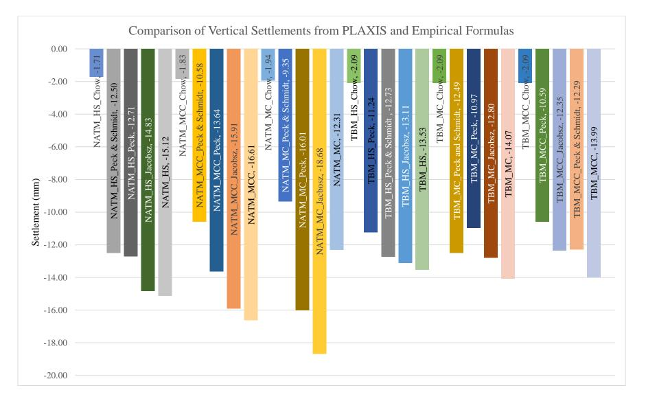
Figure 4.32: Comparison of Vertical Settlements of Different Empirical Formulas for both NATM and TBM methods (for different models)
