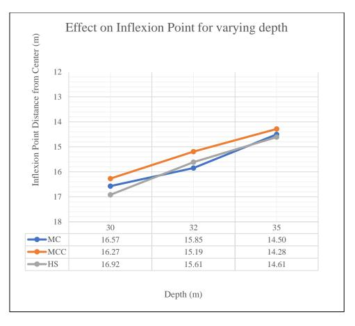
Figure 4.30: Effect on Inflexion Point for increasing of depth (30m, 32m and 35m)
