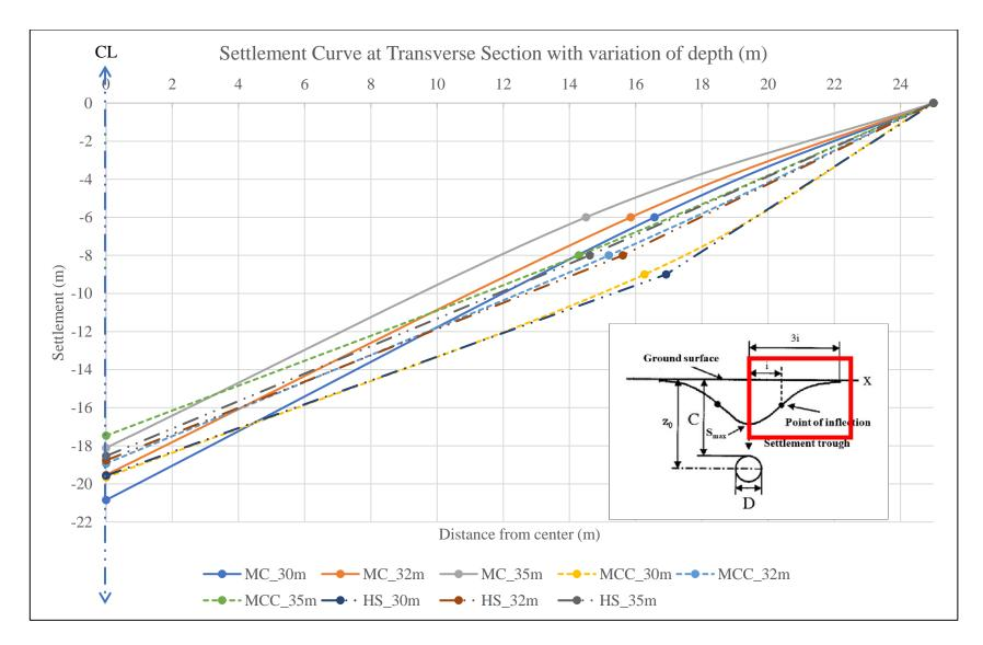
Figure 4.26: Transverse Settlement Trough Pattern with variation of depth (30m, 32m, 35m) for MC, MCC and HS Models
