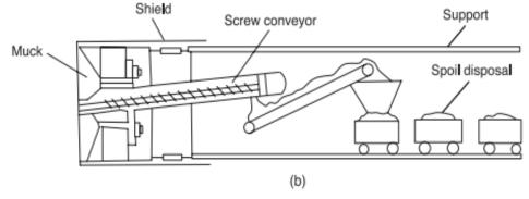
**Figure 2.11:** Conceptual Diagrams for EPB shields: (a) method to counter water and earth pressures; (b) mechanical components and arrangements in the EPB concept (Tatiya, 2005)
