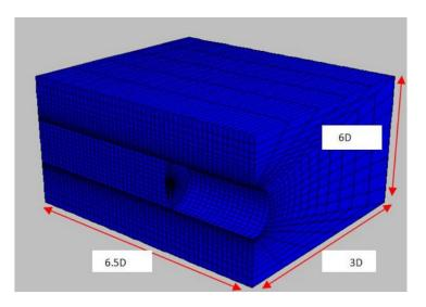
Figure 3.4: Dimension of the 3D Simulation in FLAC3D (Eslami et al., 2020)
