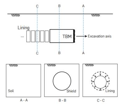
Figure 4.9: Schematic illustration of tunneling simulation process (Bentley, 2018)
