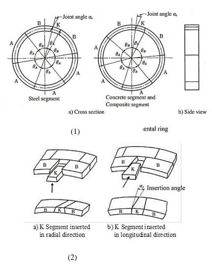
**Figure 2.19:** (1) Components of a Segmental Ring, (2) Types of K segment (Source: Internet)
