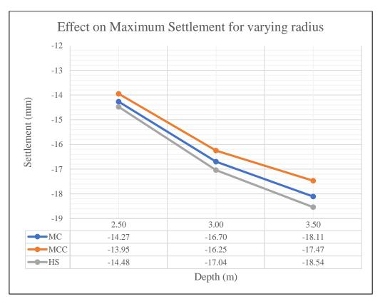
**Figure 4.29:** Effect on Maximum Settlement for increasing of radius (2.50m, 3.00m and 3.50m)
