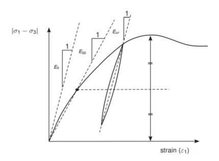
**Figure 2.37:** Definition of  $E_0$ ,  $E_{50}$  and  $E_{ur}$  for drained triaxial test results (Bentley, 2018)
