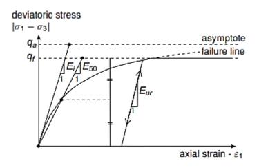
**Figure 2.38:** Hyperbolic stress strain relation in primary loading for a standard drained triaxial test (Bentley, 2018)
