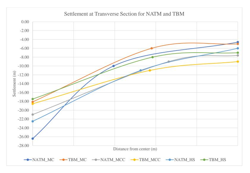
Figure 4.34: Settlement at Transverse Section for both NATM and TBM methods considering 35m depth and 3.50m radius (from PLAXIS)
