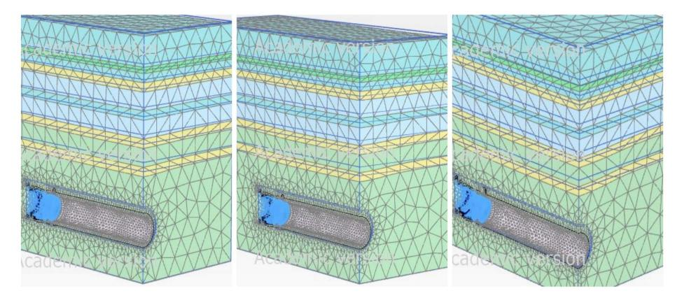
Figure 4.14: TBM Method (MC, MCC, HS model): Depth 35m and Diameter 7m
