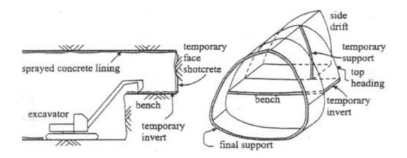
Figure 2.7: Schematic View of SCL Method (Potts, 2001)
