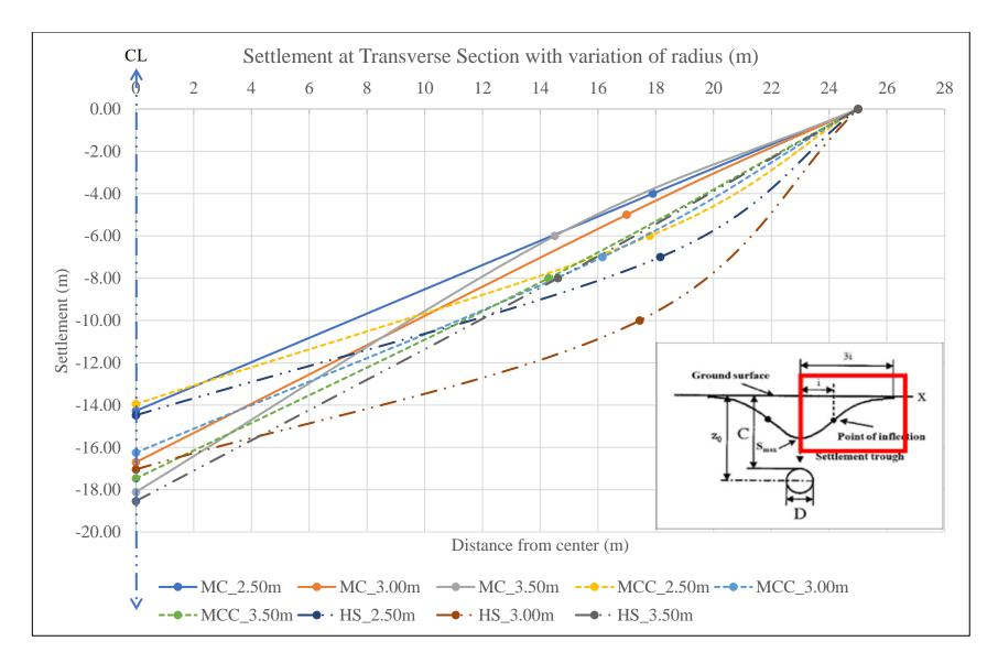
Figure 4.27: Transverse Settlement Trough Pattern with variation of radius (2.50m, 3.0m, 3.50m) for MC, MCC and HS Models
