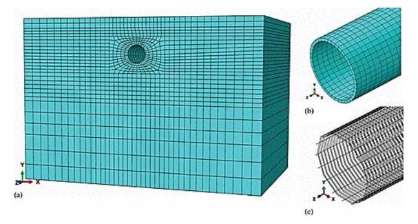
**Figure 2.30:** Typical Finite Element Model Simulation for Shield TBM Tunnel (Luo et al., 2018)
