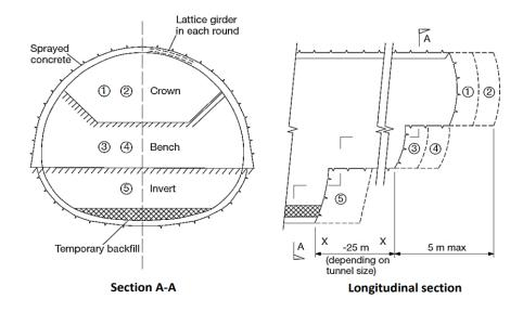
Figure 2.9: Sample Construction Sequence of Crown, Bench and Invert (ICE, 1996)
