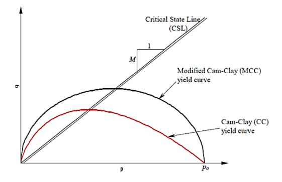
Figure 2.43: Cam Clay and Modified Cam Clay Yield Surfaces (Wood, 1990)
