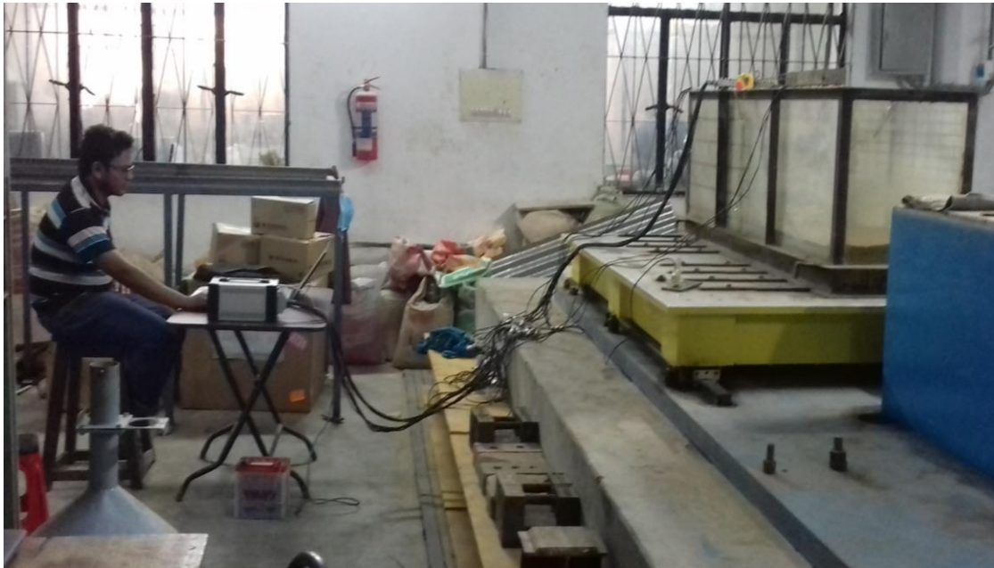
Fig. 3.29 Full Connection Set-up between the Wrap-faced Sand Retaining Wall and the Data Logger before conducting the Shake Table Testing
