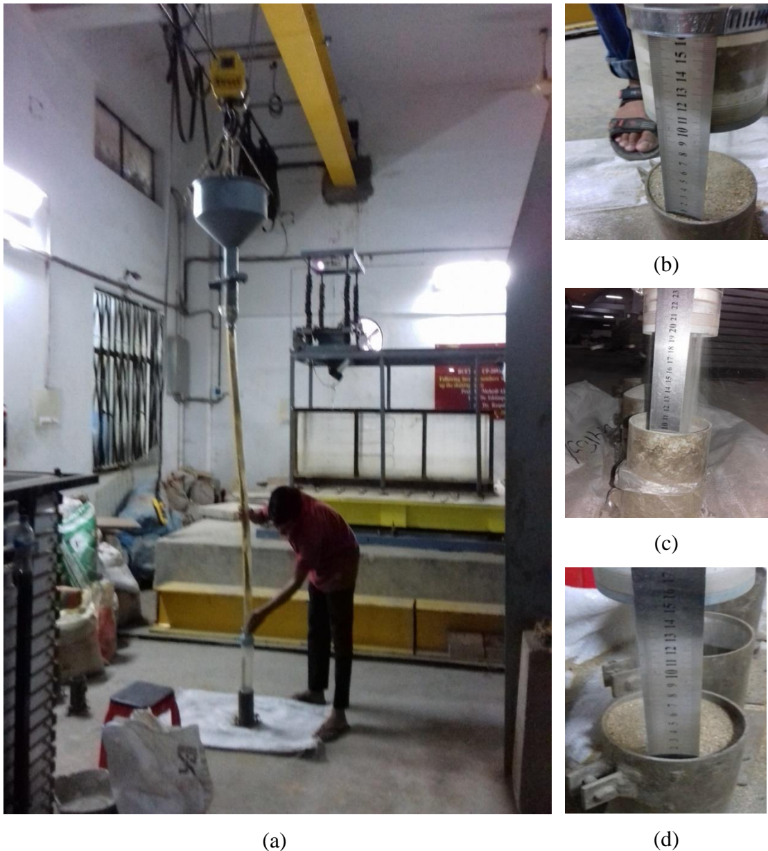
Fig. 3.14 (a) Full Experimental Set-up of a Pluviator, (b) 10 cm, (c) 20 cm and (d) 15 cm height of fall for relative density experiments
