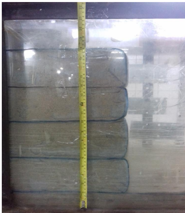
Fig. 3.31 Attachment of measuring tape with the Wrap-faced Retaining wall
