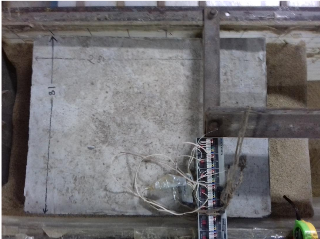
Fig. 3.32 Placement of 1.72 kPa Surcharge Load on the Retaining Wall
