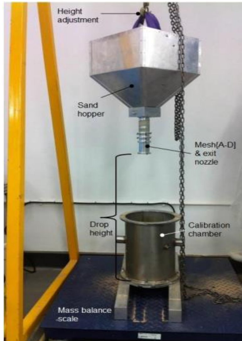
Fig. 2.18 Sand pluviation configuration. (Hakhamaneshi et al. 2016)
