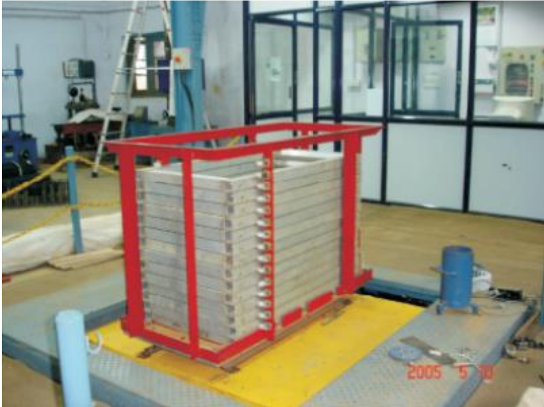
Fig. 2.21 Laminar box mounted on shaking table (Krishna and Latha 2007)
