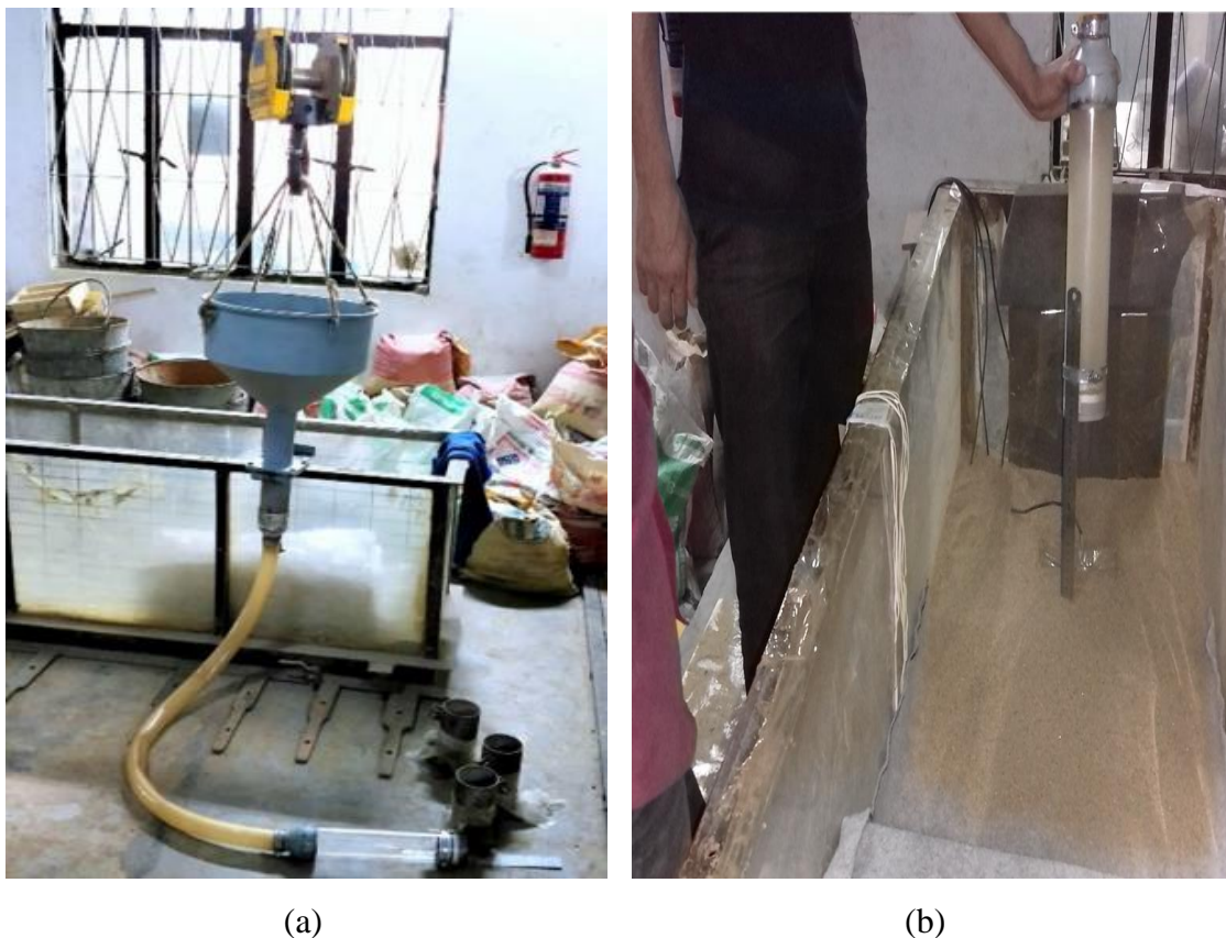
Fig. 3.21 (a) Portable Travelling Pluviator, (b) Preparation of Sand bed
