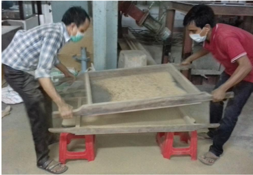
Fig. 3.3 Collection of Sylhet sand sample for Sieve No. 16 passing and Sieve No. 100 retained
