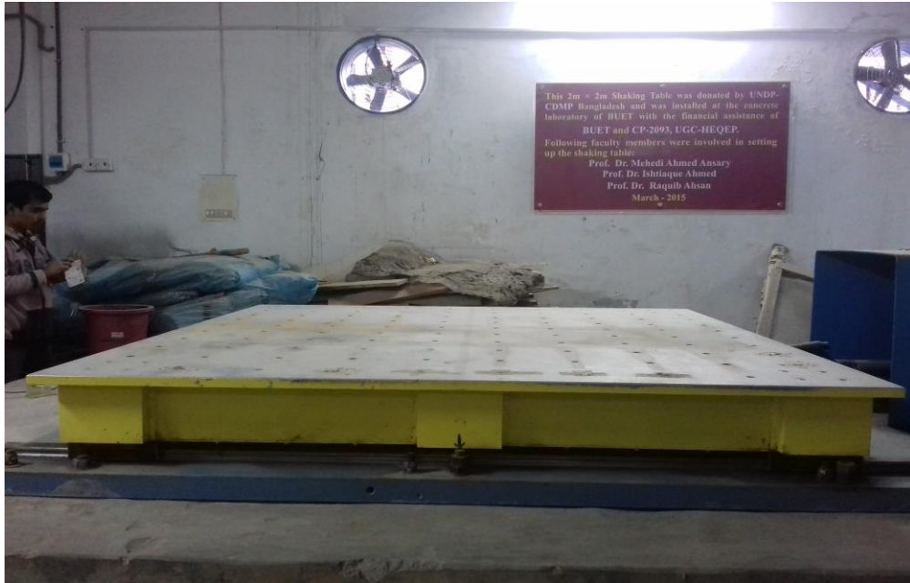
Fig. 3.18 Shake Table Facility
