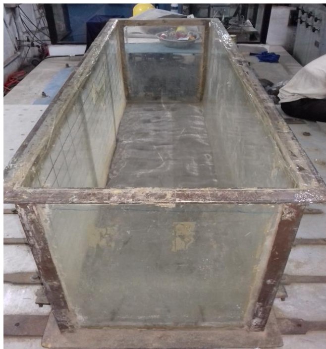
Fig. 3.19 Container for building model
