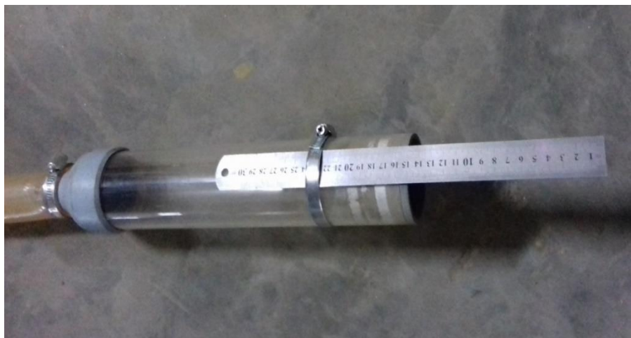
Fig. 3.11 A Reference Scale is adjusted with Rigid Tube to measure the height of fall
