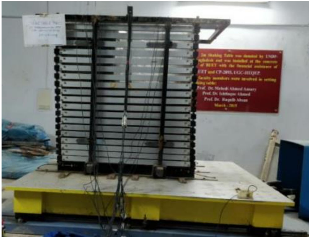
Fig. 2.22 Laminar box mounted on the shaking table (Hore et al. 2020)
