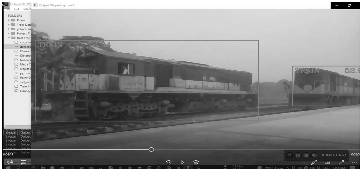
Figure 4.1 (b): Real time detection of two trains in the same frame. The frame is captured using webcam.
