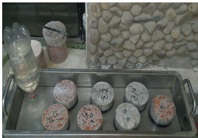
Figure 4.8: Test setup for Rate of water absorption (sorptivity)
