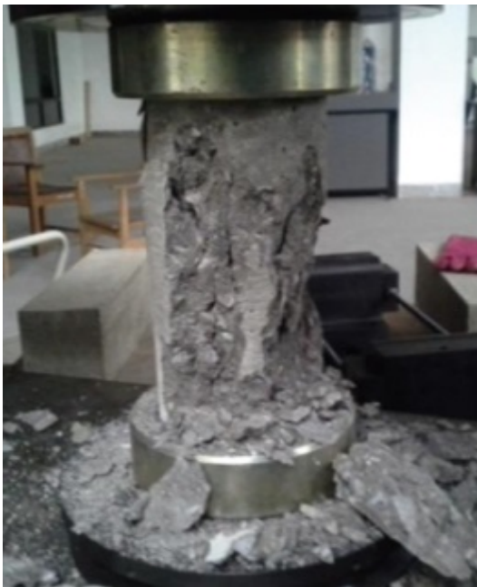
Figure 5.8: (a) Normal concrete failure
