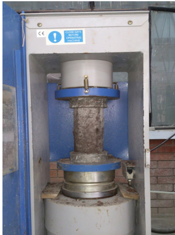
Figure 4.1: Test setup for compression test of cylinders
