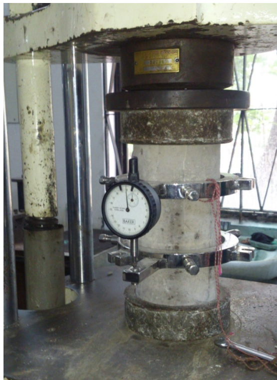
Figure 4.3: Test setup for Modulus of Elasticity
