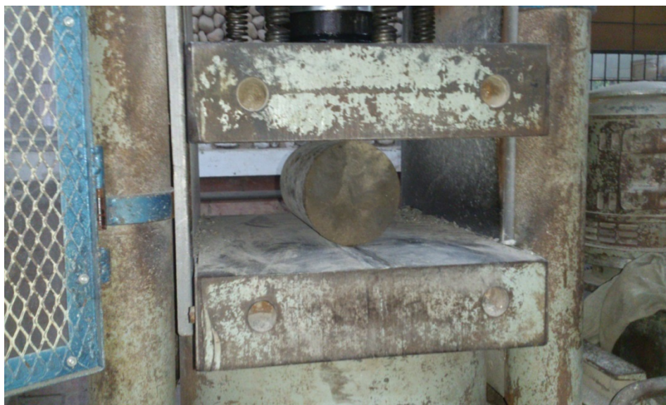
Figure 4.2: Test setup for splitting tensile strength of cylinders
