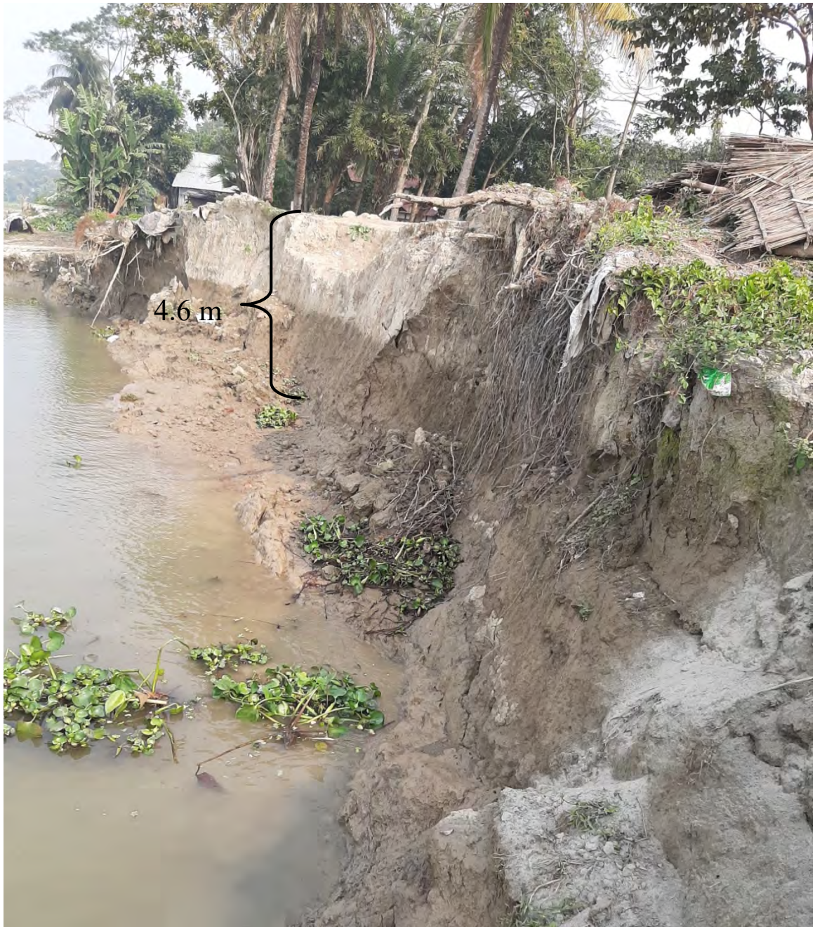
Photo D14: Photo showing the height of cut-bank of bend B22 at Kanurgau village near Khasherhat bazaar, Kalkini Upazila (N=23°06.006', E =90°20.045')
