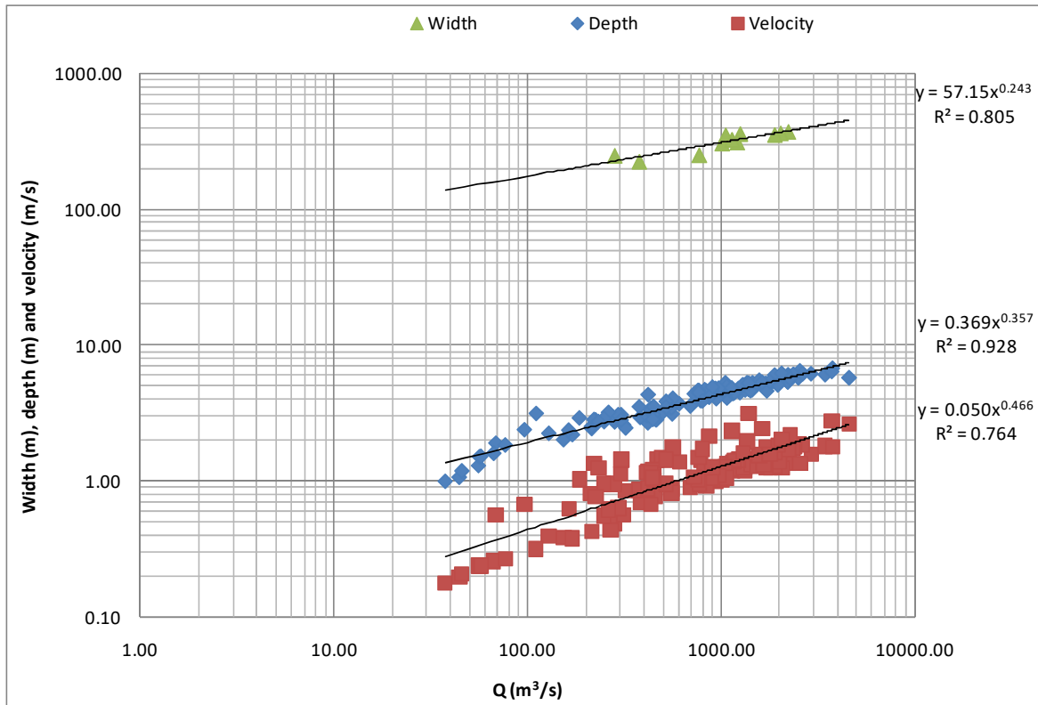
Figure 5.25: The relationship of W , D and U to changing Q at the station of the Arial Khan River offtake.
