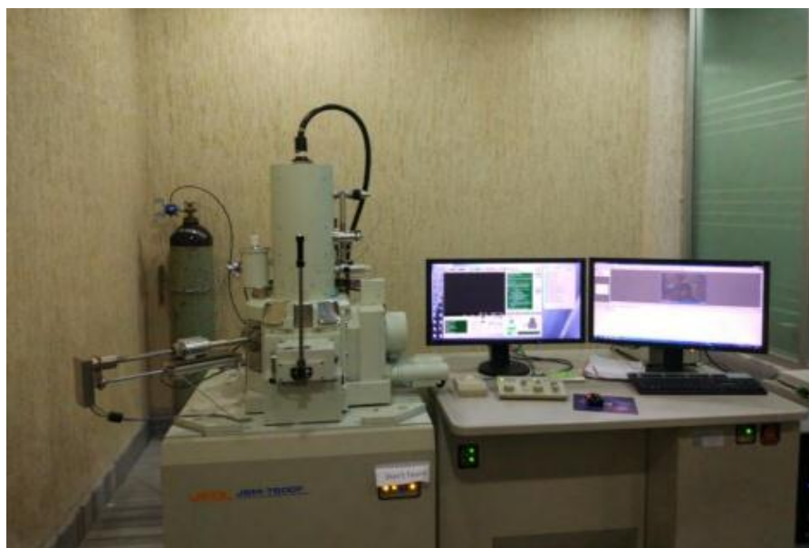
Figure 2. 2: Scanning Electron Microscopy (SEM) setup at Department of Glass and Ceramic Engineering (GCE), BUET.
