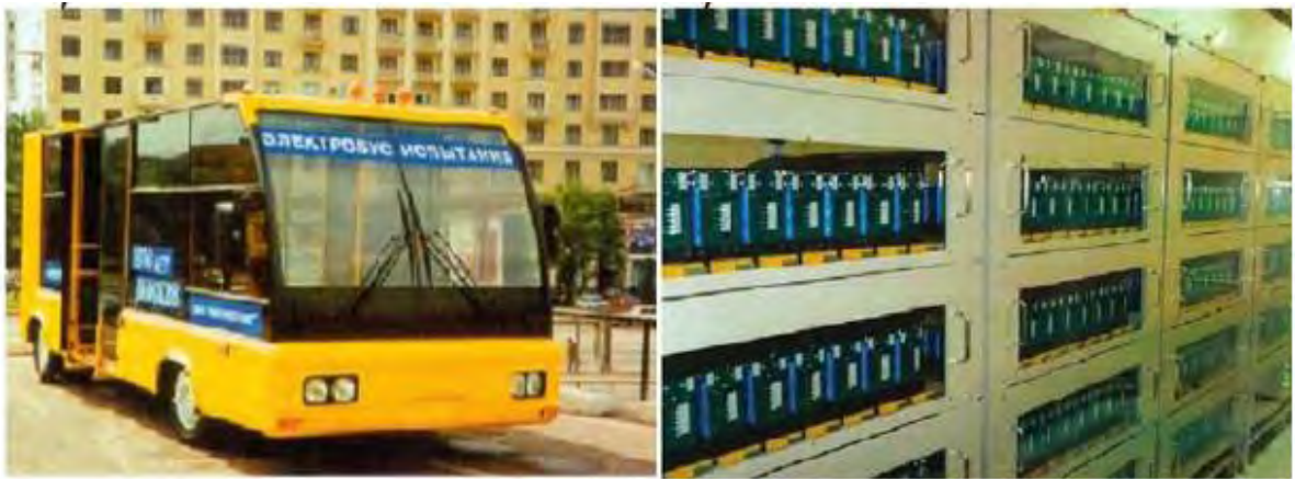
Fig 1. 5: Electric bus powered by Li-ion battery with support of supercapacitor [18].
