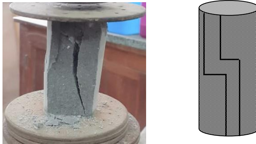
Figure 4.20: Failure pattern of 2:1 proportionate grouted sand after 120 days
