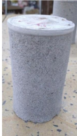
Figure 3.15: Grouted sample is retrieved from trial 4
