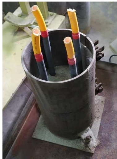
Figure 2.9: Four sleeve port pipe in a cylindrical mold to prepare grout sample
