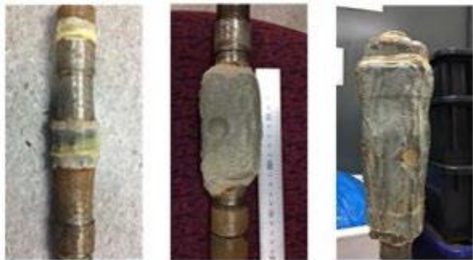
Figure 3.16: Grouting samples from laboratories setup (Carter et al., 2019)
