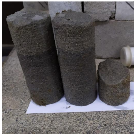
Figure 3.9: Irregular shaped sample from trial 1
