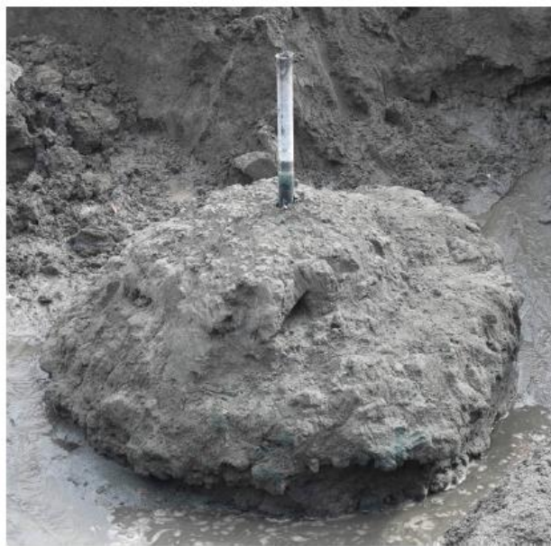
Figure 3.17: Grouting samples from field setup (Hashimoto et al., 2015)
