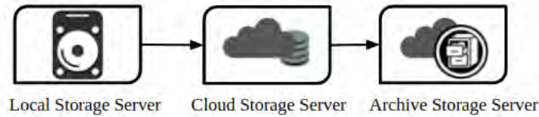
Figure 4.9: Three types of storage servers for ensuring high availability, less storage, and long-lasting archive system. Local storage server has the direct connection with CCTV camera. Cloud storage and archival storage servers are located in data centers.
