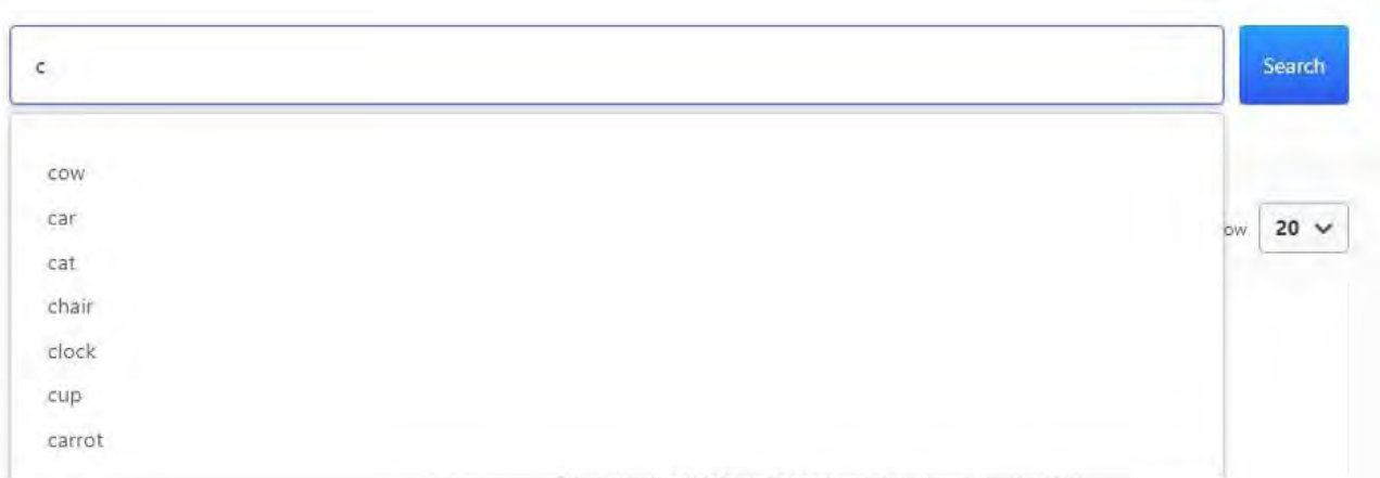
Figure 5.15: Our implemented completion suggester UI using Elasticsearch API in the backend
