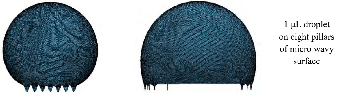
Figure 3.7: Stable simulated droplet shapes for different anisotropic configurations on micro V-grooved and micro wavy surfaces [All droplet figures are not presented at same scale here].
