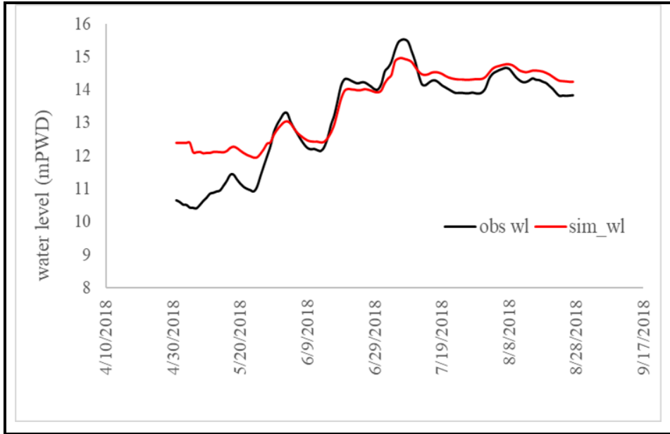
Figure 5.1 : Water level calibration at Kazipur station
