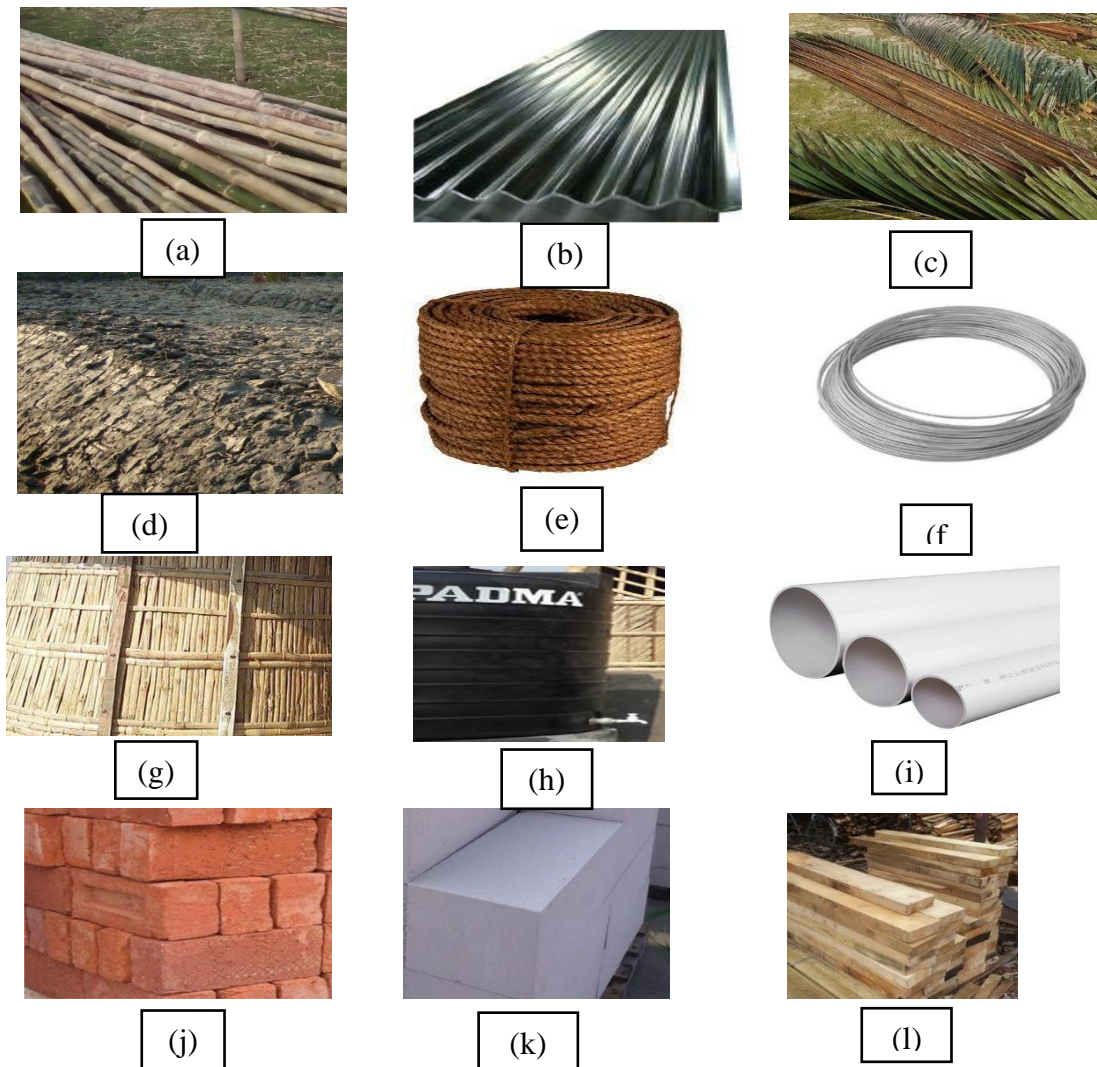
Figure 6.5: Selected materials for design implementation phase. (a) bamboo (b) CGI sheet (c) palm leaves (d) mud (e) jute rope (f) steel wire (g) bamboo matt (h) tank (i) PVC pipes (j) bricks (k) Concrete Block (l) 14 CFT wood. Source: Author and web.
