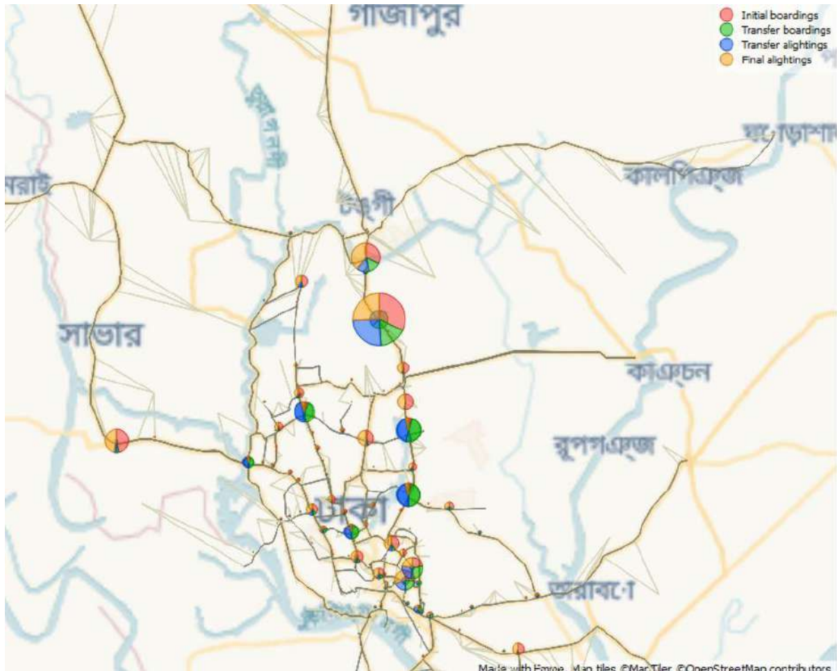
Figure 34: Distribution of passengers in MRT and rationalized bus stops for peak period of 2035 (Scenario 6)
