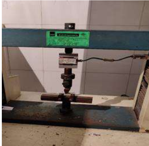
Fig. 2.9 Specimen setup for Flexural test under UTM.
