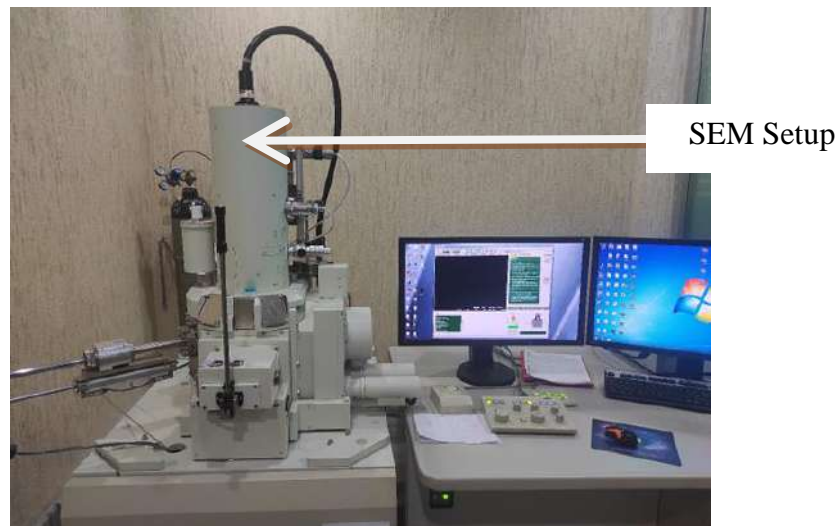
Fig. 3.12 SEM setup for measuring cutting tool wear for developed composite material under both Dry and MQL condition.
