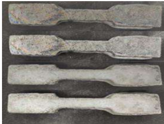
Fig. 2.6 Specimen of carbon nanotube reinforced AMMC for Tensile test.
