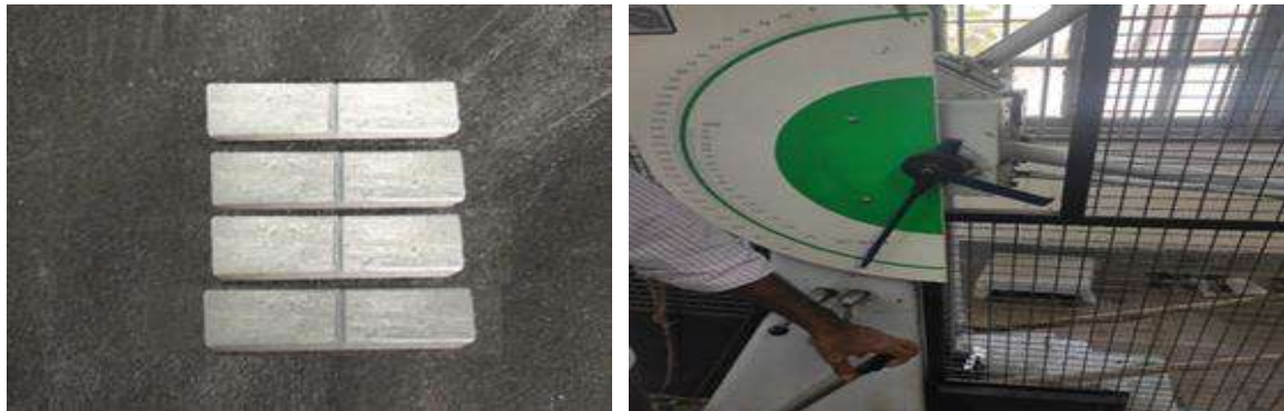
Fig. 2.11 Specimens for Impact test. Fig. 2.12 Experimental setup for Impact test.
