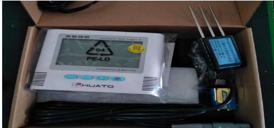
Figure 4.11 Soil moisture and temperature measurement data logger (HUATO-SS00)
