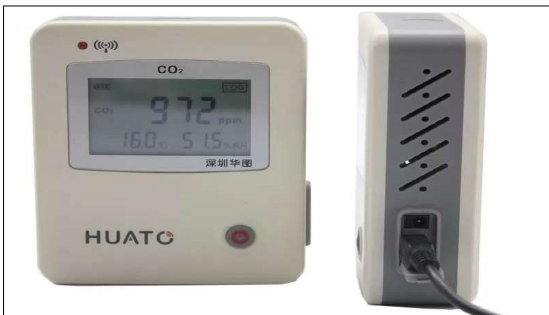
Figure 4.8 Temperature-RH-CO 2 measuring data loggers (HUATO, S653)
