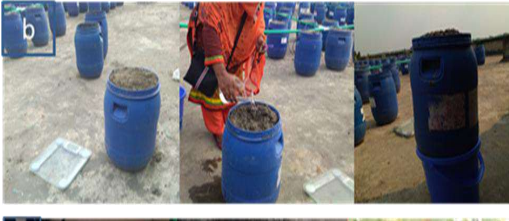
Figure 4.10 Measurement of field capacity of soil in the experimental
