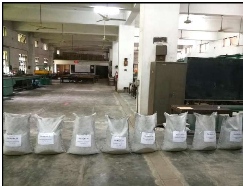
Photograph 3.10: Sand filled geobags before experiment
