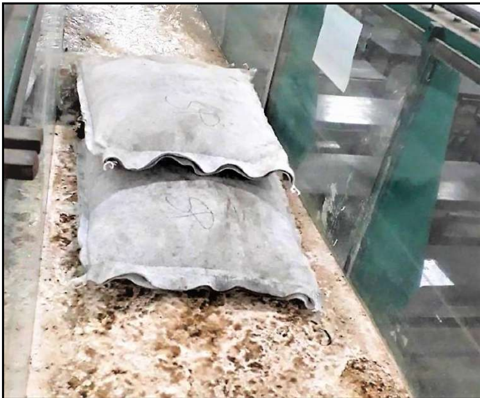
Photograph 3.15: Two layers of three geobags placed on flume (front view)
