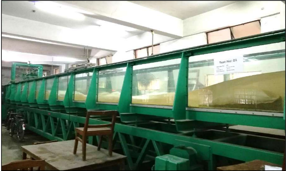
Photograph 3.4: Flume in the Hydraulic and River Engineering Laboratory
