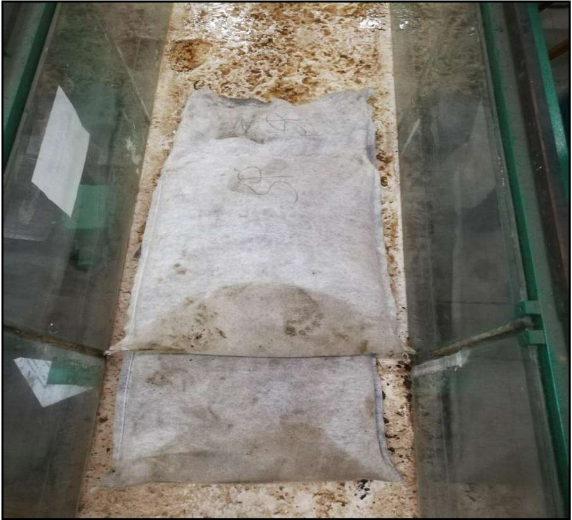
Photograph 3.16: Two layers of three geobags placed on flume (top view)
