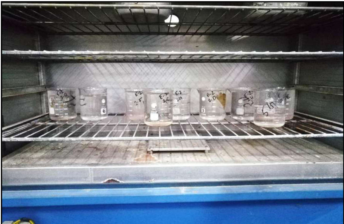
Photograph 4.7: Placement of collected sample on the oven for drying
