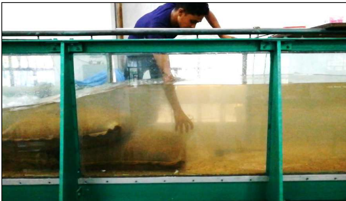
Figure 4.4: Sample collection from u/s of test section
