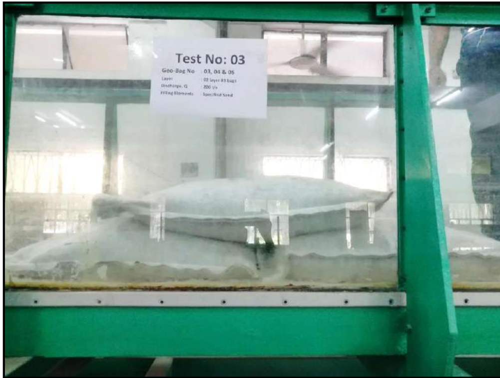
Photograph 3.14: Two layers of three geobags placed on flume (side view)
