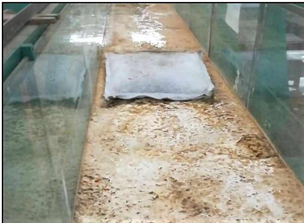
Photograph 3.13: One layer of one geobag placed on flume bed (front view)
