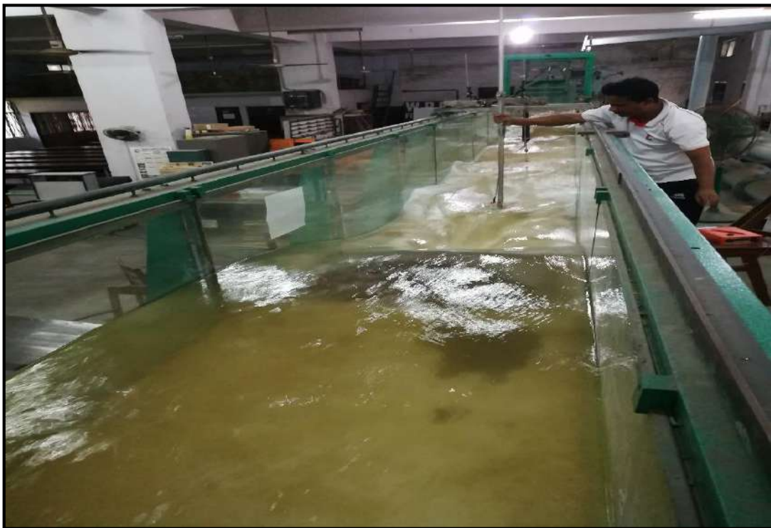
Photograph 4.2: Velocity Measurement by current meter during experimental test run
