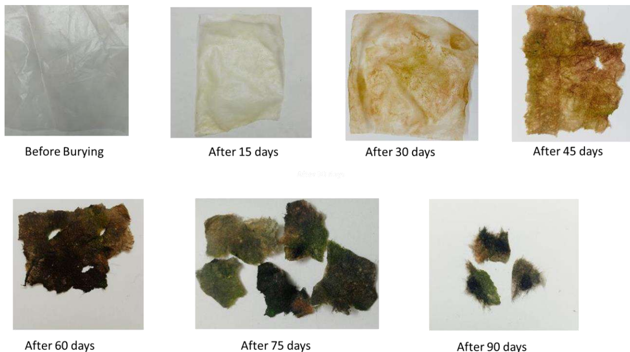
Figure 4.23 Images for various stages of film with 0.2% CC in soil burial method.
