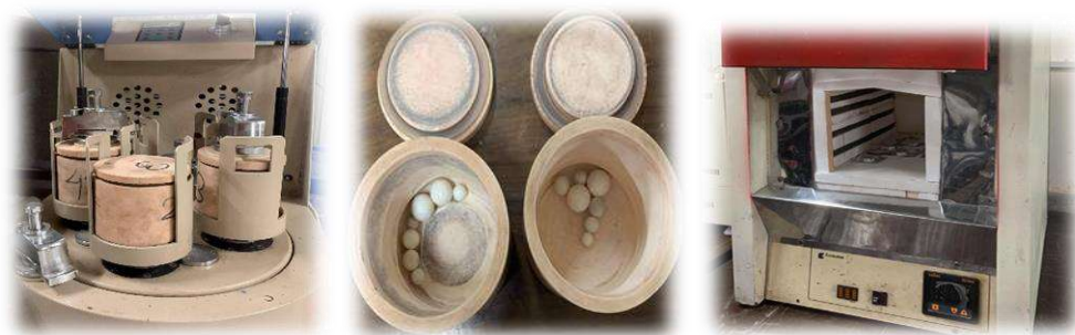
Fig 3.5: Zircon nanoparticle formation by dry ball-milling followed by annealing
