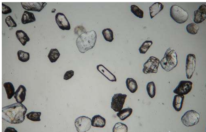
Fig 2.1: A mixture of tetragonal prism, rounded ellipsoid of zircon ( ZrSiO_4 ) sand particle
