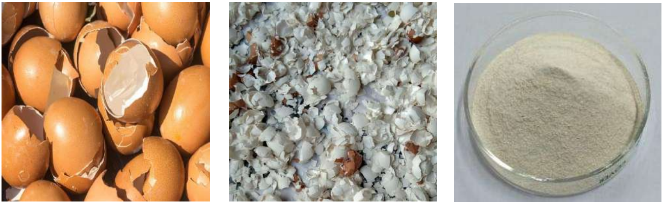
Figure 3.2: Raw eggshell collection, crushed, sieve, and preparation for calcination
