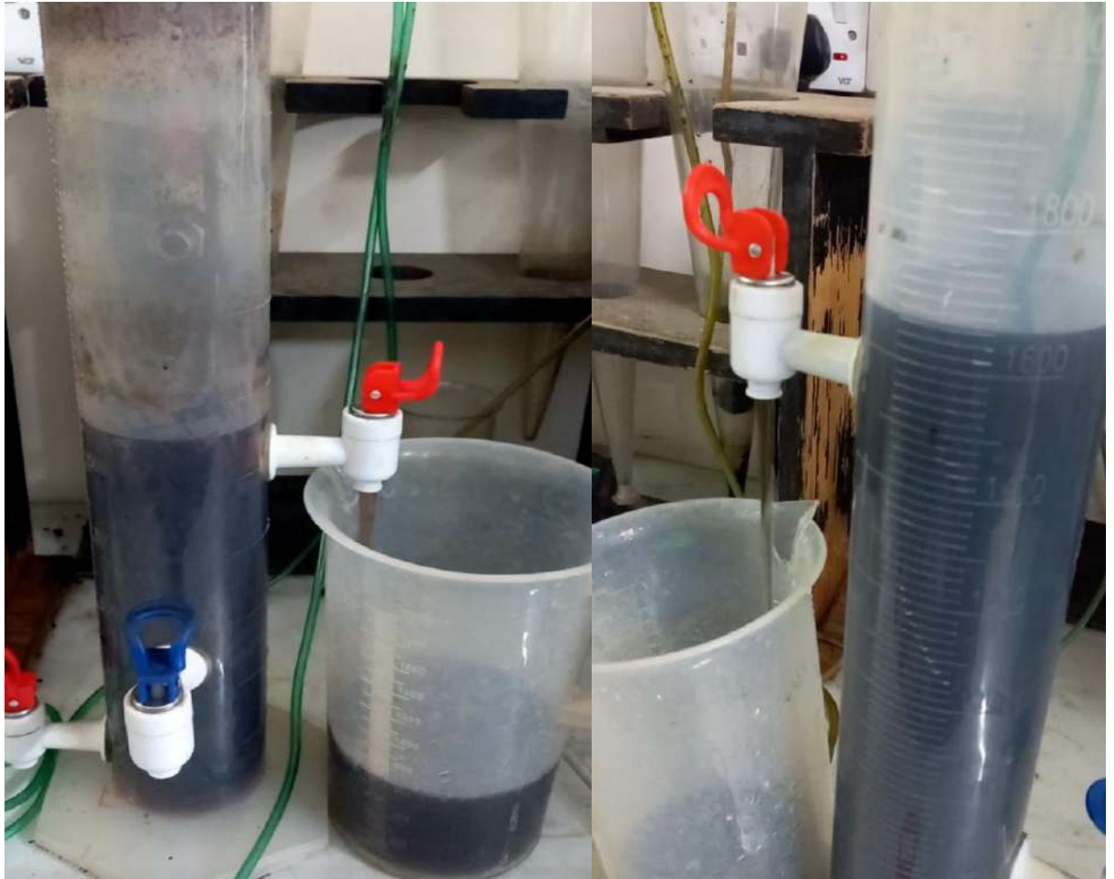
Figure 3.18: SBR cycle decanting steps during An-Ae SBR operation for treatment of RTWW
