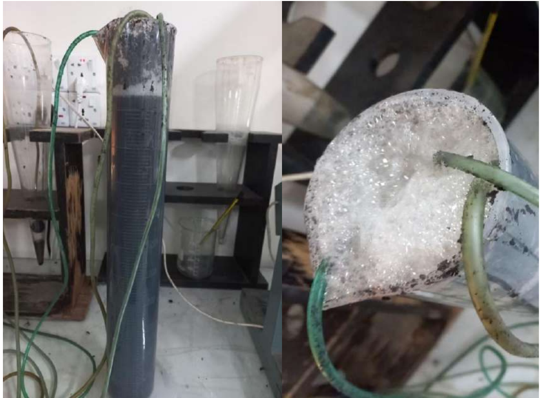
Figure 3.17: SBR cycle aeration steps during An-Ae SBR operation for RTWW treatment
