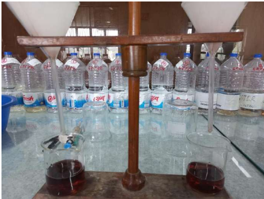
Figure 3.6: Gravity filtration for TDS measurement
