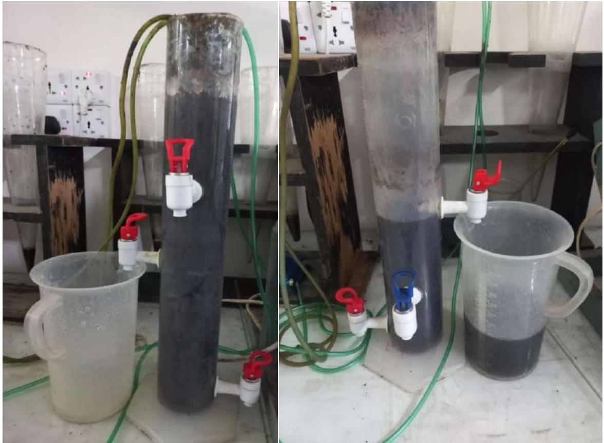
Figure 3.14: SBR cycle decanting step during granulation phase of the study
