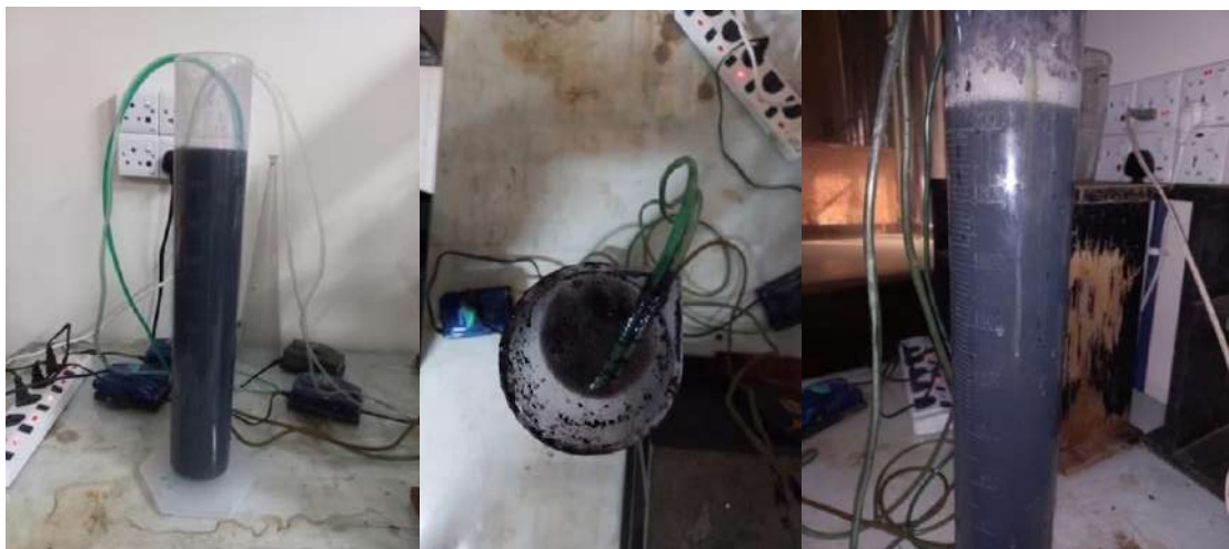
Figure 3.11: SBR Cycle aeration-reaction step during granulation phase of the study
