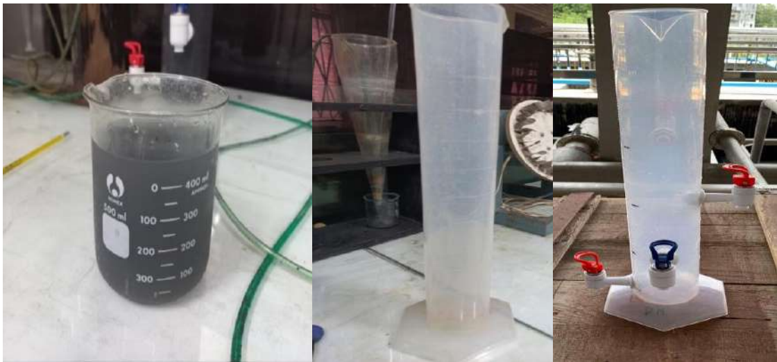
Figure 3.7: RTWW in beaker and measuring cylinder as SBR Reactor
