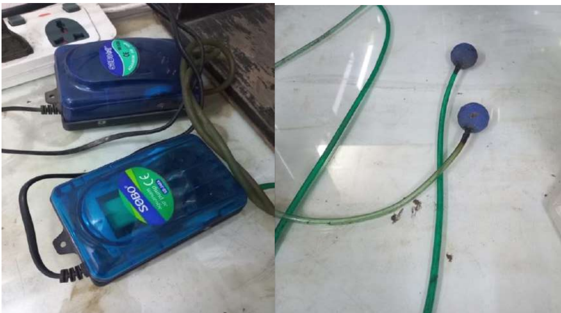
Figure 3.8: Air Blower/Aerator and Air Diffusers (Ceramic Type-Stone shaped)
