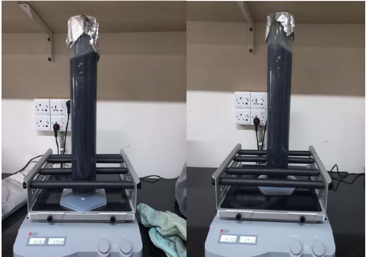
Figure 3.16: SBR cycle anaerobic step during An-Ae SBR operation for treatment of RTWW
