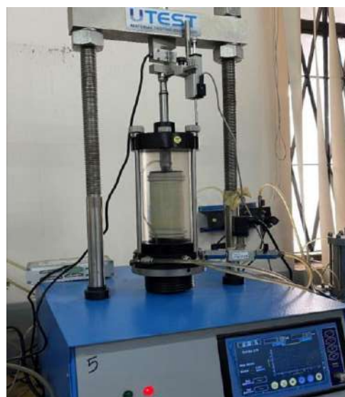
Figure 3.3: Triaxial test setup
