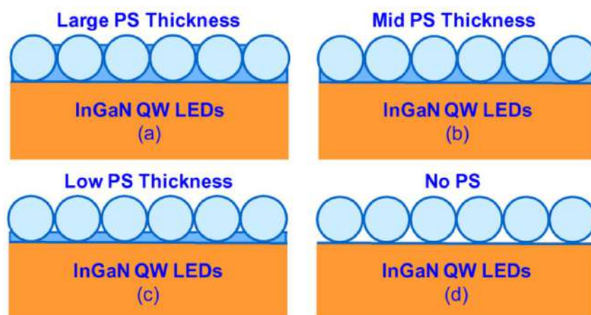
Figure 2.3: (a)-(d) Schematics of InGaN QW LEDs with \text{SiO}_2 / Polystyrene (PS) microlens array where PS thickness is varied [71].
