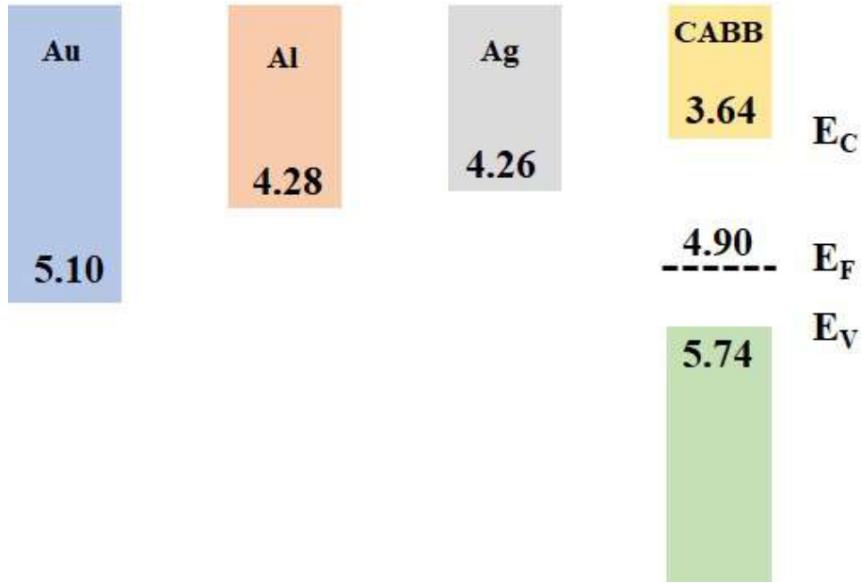
Figure 4.5: The energy level diagram of the \text{Cs}_2\text{AgBiBr}_6 single crystal and different electrodes (Au, Ag, and Al).
