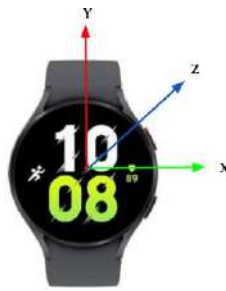
Figure 7.7: The three axes of a smartwatch
